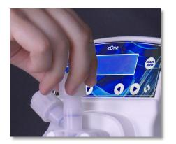
**Step 21:** Remove the Discharge Valve tube nut, collar, and nozzle. Set all three aside.
