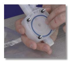
**Step 16:** Insert the large, blue o-ring into the groove on the backside of the Pump Head.
