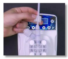
**Step 29:** Attach the tube, and tube connections onto the Discharge Valve by hand tightening the tube nut. Do not cross thread nor overtighten.
