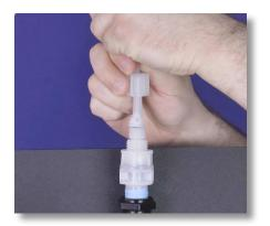
**Step 36:** Attach the tube, and tube connections onto the Injection Valve by hand tightening the tube nut. Do not cross thread nor overtighten.
