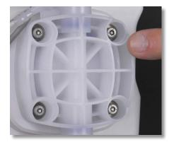
Step 3: Locate the Pump Head screws.
