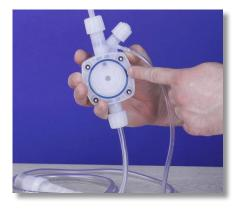
**Step 8:** Once removed, check the backside of the pump head to see if the blue o-ring is in the groove.
