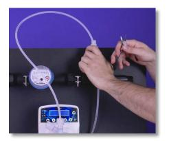
**Step 33:** Grab the rigid polyethylene Discharge tube connected to the Discharge Valve. Using diagonal pliers or cutters, cut the tube so that it runs comfortably from the discharge valve to the Injection Valve.
