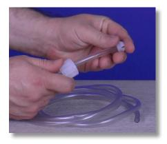
**Step 40:** Attach the tubing connections onto one end of the PVC tube, be mindful of their orientation.
