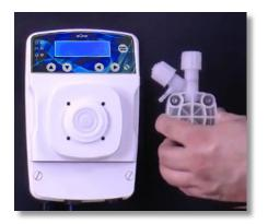
**Step 17:** To install the new Pump Head, align it so that the Y-shape points upward on the **eOne** pump.
