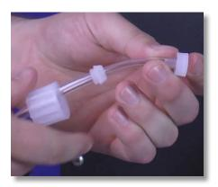
**Step 53:** Grab the PVC Suction tubing hanging down from the Suction Valve, and attach the tube connections onto the loose end of the PVC Suction tubing. Be mindful of the orientation for the tubing connections.
