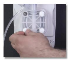
**Step 2:** In order to remove the Pump Head, use your finger or a flat blade screwdriver and take off the four white caps at the corners of the Pump Head.
