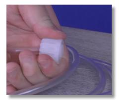
**Step 41:** Push the collar and nozzle together as close as possible. Pull the tube nut toward the nozzle to compress the collar and nozzle tight together, forming a ferrule connection.
