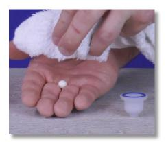
**Step 48:** Pour the ceramic ball out of the filter seat and into your hand and use the small towel to wipe the ceramic ball clean. Do not misplace it.
