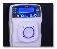
**Step 9:** If the blue o-ring is not there, still discard the Pump Head and connected items, but check to see if the blue o-ring is stuck to the **eOne** pump.
