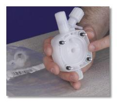
**Step 15:** Take the new Pump Head out of its bag, and turn it over so you are looking at the backside of the pump head.
