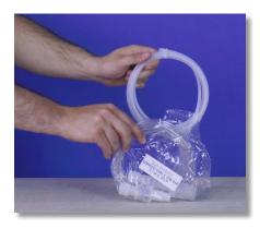
**Step 23:** Open the Tubing Kit and take out the rigid polyethylene Discharge tubing. Set the Tubing Kit aside.
