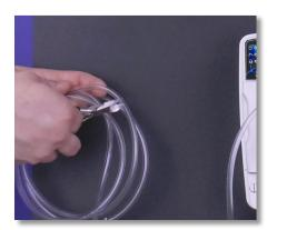
**Step 60:** Using the diagonal pliers, cut the tube so that it is long enough for the chemical bleed off to go into the bucket or stock tank while priming the **eOne** pump.
