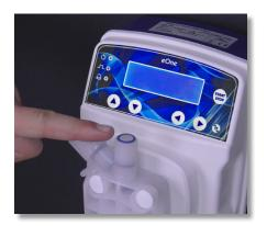
**Step 22:** Make sure not to lose the blue o-ring underneath the tube nozzle and sitting on the Discharge Valve.
