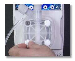
Part 4c - If the pump draws chemistry but does not inject, tighten the Pump Head:
