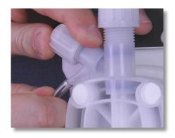
**Step 21:** Remove the bleed-off tubing from the Air Bleed Barb and set it outside of the chemical bucket.
