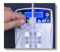
**Step 25:** Now close the Air Bleed Valve by turning it clockwise.
