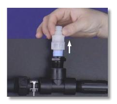
**Step 8:** Locate and remove the Injection Valve from the installation saddle or tee. Visually inspect the Injection Valve for debris. Try to clear the debris with either running water or using a seal pick.
