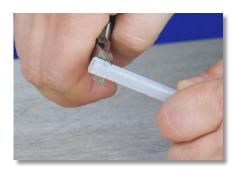
**Step 7:** Visually inspect the condition of the rigid polyethylene Discharge Tubing. If either end of the tubing is flared, use the diagonal pliers to cut the flared portion off. If the tubing is cracked, old, or broken, then you need to replace it now.
