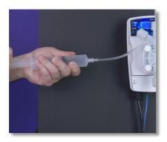
**Step 22:** Using the Syringe Kit, slide the 4mm adapter of the syringe onto the Air Bleed Barb and draw the plunger back. Chemistry should enter the syringe. This may take a couple of tries.
