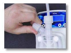
Part 4a - If the pump draws chemistry but does not inject, check the Air Bleed Valve:
