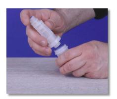
**Step 29:** Insert the filter basket into the filter body and forcefully pop them together.
