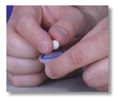
**Step 26:** Put the ceramic ball back into the filter seat and set the filter seat aside.
