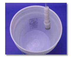
**Step 6:** Lift the PVC Suction Tubing, along with the Foot Filter out of the chemical bucket or stock tank.
