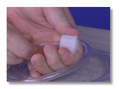
**Step 16:** Push the Collar and Nozzle together as close as possible, and pull the Tube Nut toward the Nozzle to compress the Collar and Nozzle tight together, forming a ferrule connection.
