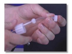
**Step 11:** Remove the Nozzle, Collar, and Tube Nut from the PVC Suction Tube and set aside. Do not lose them.
