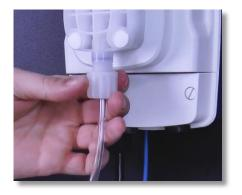
**Step 17:** Reattach the tube and tubing connections onto the Suction Valve of the Pump Head by hand tightening the Tube Nut. Do not cross thread or overtighten.
