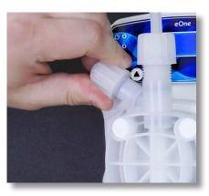
**Step 37:** Locate the Air Bleed Valve on the upper left portion of the Pump Head and open it by turning the valve counter-clockwise.
