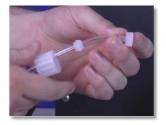
**Step 8:** Remove the Nozzle, Collar, and Tube Nut from the PVC Suction Tubing and set aside. Do not lose them.
