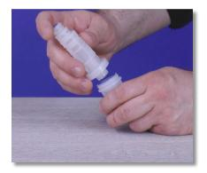
**Step 20:** If not, separate the Foot Filter into three (3) pieces by popping the filter basket from the filter body.
