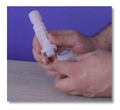
**Step 21:** The filter seat may stick to the filter body. Make sure the filter seat rests in the filter basket to avoid losing the ceramic ball.
