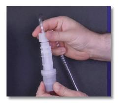
**Step 31:** Grab the PVC Suction Tubing and Connections hanging from the Suction Valve of the pump. Reattach the Tubing Connections to the Foot Filter by hand tightening the Tube Nut. Do not cross thread or overtighten. Make sure the Foot Filter Nipple O-Ring is properly seated.
