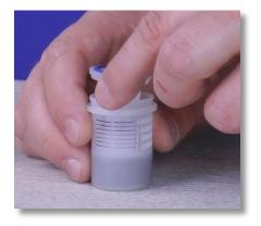
**Step 28:** Set the filter body down, grab the filter basket and put the filter seat back into the filter basket.
