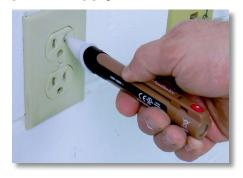
**Step 1:** First, check if the breaker is off. If the breaker is on, the outlet could be bad.
