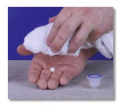
**Step 24:** Pour the ceramic ball out of the filter seat and into your hand. Set the filter seat down and use the small towel to wipe the ceramic ball clean. Do not misplace it.
