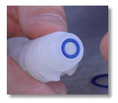
**Step 27:** Grab the filter body and inspect to make sure the small blue o-ring on top of the filter body is not damaged.
