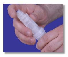
**Step 30:** Pull on the two (2) sections to make sure they are connected securely and shake the Foot Filter back and forth once more, verifying the ceramic ball is moving freely.
