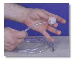
**Step 14:** Grab the Suction Valve Tube Nut and slide one end of the flexible PVC Suction Tubing through the outside opening of the Tube Nut.
