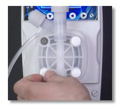
**Step 33:** Over time, the Pump Head may work itself loose from the pump. To check this, remove the four (4) white screw caps on the pump head.
