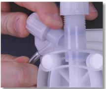
**Step 38:** Remove the Bleed-Off Tubing from the Air Bleed Barb and set it outside of the chemical bucket.
