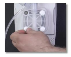
**Step 2:** In order to remove the Pump Head, use your finger or a flat blade screwdriver and take off the four white caps at the corners of the Pump Head.
