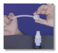
**Step 34:** Re-attach the tube connections onto the loose end of the connected Discharge Tubing. Be mindful of their orientation for the tubing connections.
