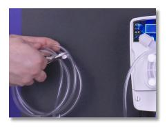
**Step 60:** Using the diagonal pliers, cut the tube so that it is long enough for the chemical bleed off to go into the bucket or stock tank while priming the **eOne MF** pump.
