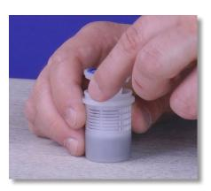
**Step 50:** Place the filter seat back into the filter basket.
