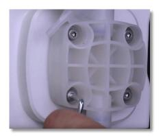
**Step 18:** Use the Allen wrench to carefully hand-tighten the four (4) Pump Head screws in a crisscross pattern until evenly snug.
