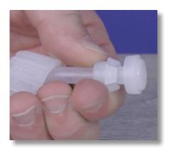
**Step 27:** Push the collar and nozzle together as close as possible.
