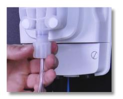
**Step 42:** Attach the tube, and tube connections onto the Suction Valve by hand tightening the tube nut. Do not cross thread nor overtighten.
