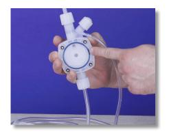
**Step 8:** Once removed, check the backside of the Pump Head to see if the blue o-ring is in the groove.
