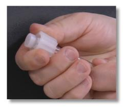
**Step 55:** Pull the tube nut toward the nozzle to compress the collar and nozzle tight together, forming a ferrule connection.
