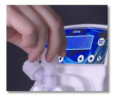
**Step 21:** Remove the Discharge Valve tube nut, collar, and nozzle. Set all three aside.
