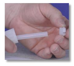
**Step 25:** Slide the collar onto the tube, and make sure the collar's crown is pointing away from the tube nut.
