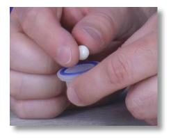
**Step 49:** Put the ceramic ball back into the filter seat.
