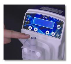
**Step 22:** Make sure not to lose the blue o-ring underneath the tube nozzle and sitting on the Discharge Valve.
