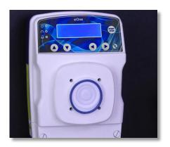
**Step 9:** If the blue o-ring is not there, still discard the Pump Head and connected items, but check to see if the blue o-ring is stuck to the **eOne MF** pump.
