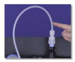
**Step 5:** Locate the used rigid Discharge Tubing connected to the old Injection Valve.
