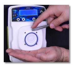
**Step 10:** If so, remove and discard the blue o-ring now. This can be done with your finger or flat blade screwdriver.
