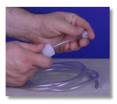
**Step 40:** Attach the tubing connections onto one end of the PVC Tube, be mindful of their orientation.
