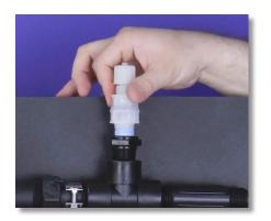
**Step 12:** Unscrew, disconnect, and discard the old Injection Valve from the installation saddle or tee.
