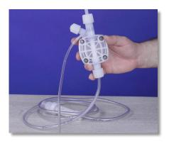
**Step 7:** Set the diagonal pliers down and use the same hand to remove the Pump Head along with the connected tubing and Foot Filter. They should all come off as one piece.
