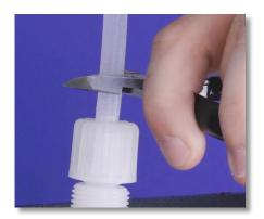
**Step 6:** Use the diagonal pliers or cutters to cut the tube as close to the old Injection Valve as possible.
