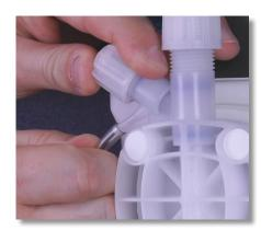
**Step 59:** Locate the manual air bleed barb on the upper left section of the Pump Head and slide one end of the PVC Tubing over the barb.
