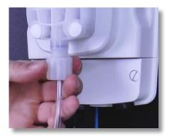
**Step 42:** Attach the tube, and tube connections onto the Suction Valve by hand tightening the tube nut. Do not cross thread nor overtighten.
