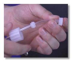
**Step 53:** Grab the PVC Suction Tubing hanging down from the Suction Valve, and attach the tube connections onto the loose end of the PVC Suction Tubing. Be mindful of the orientation for the tubing connections.
