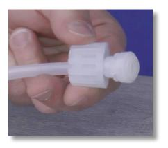
**Step 28:** Pull the tube nut toward the nozzle to compress the collar and nozzle tight together, forming a ferrule connection.
