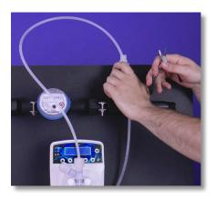
**Step 33:** Grab the rigid polyethylene Discharge tube connected to the Discharge Valve. Using diagonal pliers or cutters, cut the rigid, polyethylene Discharge Tubing to a longer length, allowing slack between the Discharge Valve and Injection Valve.
