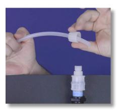
**Step 34:** Re-attach the tube connections onto the loose end of the connected Discharge Tubing. Be mindful of their orientation for the tubing connections.
