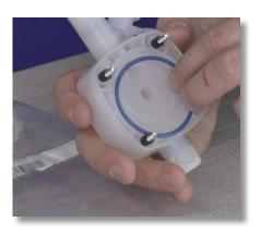
**Step 16:** Insert the large, blue o-ring into the groove on the backside of the Pump Head.
