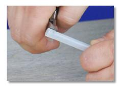
**Step 7:** Cut the rigid polyethylene discharge tubing so that it runs comfortably from the discharge valve to the injection valve. Set the remaining tubing aside.
