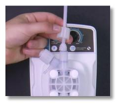
**Step 16:** Reattach the tube onto the discharge valve by hand tightening the tube nut. Do not cross thread nor overtighten.
