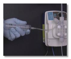
**Step 22:** Using the syringe kit, slide the 4mm adapter of the syringe onto the air bleed barb and draw the plunger back. Chemistry should enter the syringe. This may take a couple of tries.
