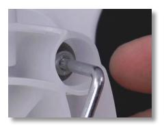
**Step 18:** Underneath the caps are four (4) pump head screws. Using the three millimeter Allen wrench, tighten the four (4) screws about 1/8 turn. It's best to tighten in a crisscross pattern.
