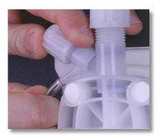
**Step 24:** Slide the bleed-off tubing back onto the air bleed barb and place the tubing back into the chemical bucket.
