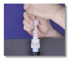
**Step 13:** Reattach the tube to the injection valve by hand tightening the tube nut. Do not cross thread or overtighten.
