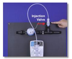
Part 4b - If the eMP draws chemistry but does not inject, inspect the Discharge Tubing, Tubing Connections, and Injection Valve:
