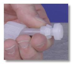
**Step 6:** Remove the connections, and set them aside. Visually inspect the condition of the rigid polyethylene discharge tubing.
