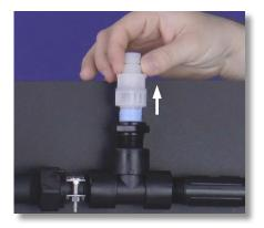
**Step 8:** Locate and remove the injection valve from the installation saddle or tee. Visually inspect the injection valve for debris. Try to clear the debris with either running water or using a seal pick.
