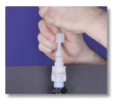
Step 3: Unscrew the tube nut from the injection valve.
