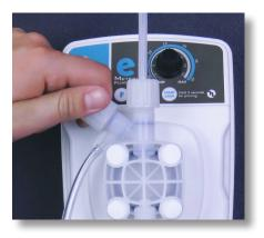
Step 25: Now close the air bleed valve by turning it clockwise.
