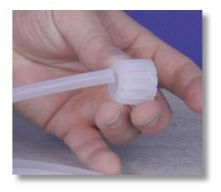
**Step 20:** Slide one end of the rigid polyethylene discharge tubing through the outside opening of the tube nut.
