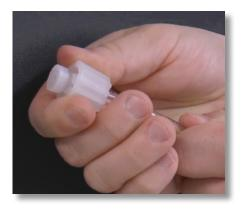
**Step 54:** Pull the tube nut toward the nozzle to compress the collar and nozzle tight together, forming a ferrule connection.
