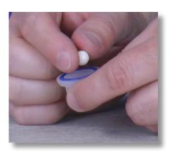
**Step 60:** Put the ceramic ball back into the filter seat.
