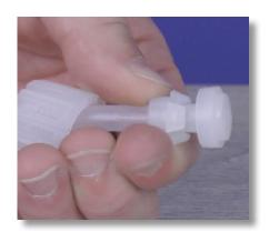
**Step 46:** Push the collar and nozzle together as close as possible.
