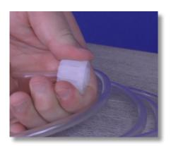
**Step 33:** Pull the tube nut toward the nozzle to compress the collar and nozzle tight together, forming a ferrule connection.
