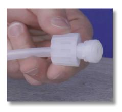
**Step 47:** Pull the tube nut toward the nozzle to compress the collar and nozzle tight together, forming a ferrule connection.
