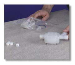
**Step 13:** Take the new pump head out of its bag along with the four (4), new, small white caps. Set the white caps aside.
