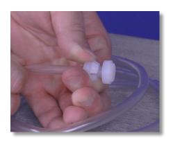
**Step 32:** Push the collar and nozzle together as close as possible.
