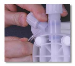
**Step 66:** Locate the manual air bleed barb on the upper left section of the pump head and slide one end of the PVC tubing over the barb.
