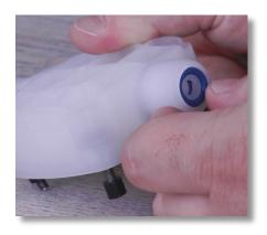
**Step 34:** Place the small blue o-ring onto the suction valve.
