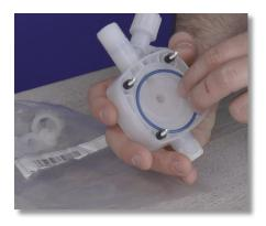
**Step 15:** Insert the large blue o-ring into the groove on the backside of the pump head.
