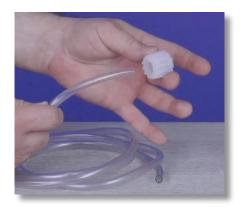
**Step 29:** Slide one end of the PVC tubing through the outside opening of your tube nut.
