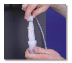
**Step 63:** Grab the PVC suction tubing hanging down from the suction valve and attach the tube, foot filter tube nut, collar, and nozzle onto the foot filter by hand tightening the tube nut. Do not cross thread nor overtighten.
