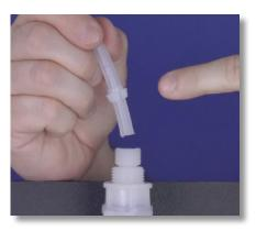
**Step 44:** Slide the collar onto the tube, making sure the collar's crown is pointing toward the injection valve.
