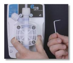
**Step 37:** Use the Allen Wrench to carefully hand-tighten the four Pump Head screws in a crisscross pattern until evenly snug. Do not overtighten. This keeps the head aligned and on straight.
