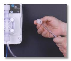
**Step 51:** Slide the open end of the PVC tubing through the outside opening of the tube nut.
