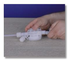
**Step 35:** Attach the tube, and tube connections onto the suction valve by hand tightening the tube nut. Do not cross thread nor overtighten.
