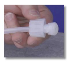
**Step 23:** Push the collar and nozzle together as close as possible, and pull the tube nut toward the nozzle to compress the collar and nozzle tight together, forming a ferrule connection.
