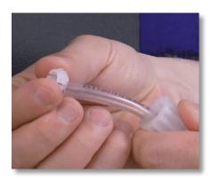
**Step 52:** Slide the collar onto the tube and make sure the collar's crown is pointing toward the foot filter.
