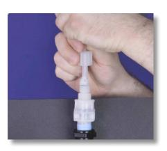
**Step 48:** Attach the tube, and tube connections onto the injection valve by hand tightening the tube nut. Do not cross thread nor overtighten.
