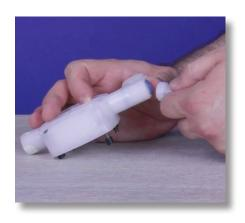
**Step 25:** Attach the tube, and tube connections onto the discharge valve by hand tightening the tube nut. Do not cross thread nor overtighten.
