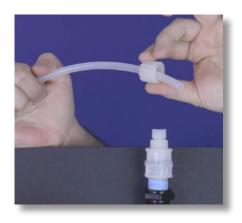
**Step 43:** Grab the injection valve tube nut and slide the loose end of the connected discharge tubing through the outside opening of the tube nut.
