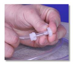
**Step 31:** Take the nozzle and insert the pointed end into the opening of the same tube.
