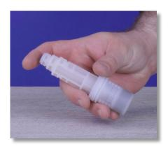
**Step 55:** Grab the foot filter and shake it back and forth. You should hear a ceramic ball moving freely inside.
