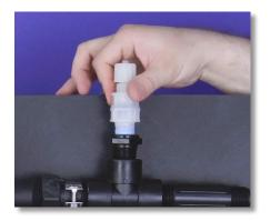
**Step 12:** Unscrew, and disconnect the old injection valve from the tee.
