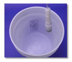
**Step 64:** Place the foot filter into the bucket or stock tank. This ensures the foot filter draws chemistry once you begin operation.
