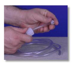
**Step 30:** Slide the collar onto the tube and make sure the collar's crown is pointing away from the tube nut.
