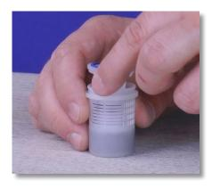
**Step 58:** Pull the filter seat out of the filter basket and set the filter basket aside.
