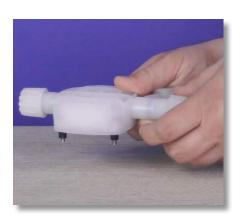
**Step 18:** If the discharge valve connections are already attached to the pump head, then remove the discharge valve tube nut, collar, and nozzle from the discharge valve at the top of the pump head.
