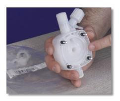
**Step 14:** Turn the pump head over so you are looking at the backside of the pump head. Check to see if the large blue o-ring sits in the groove.
