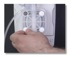
**Step 2:** First, remove and discard the four (4) white caps at the corners of the pump head.
