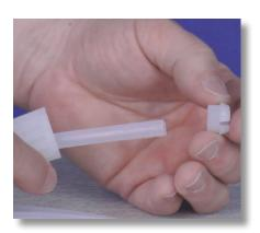
**Step 21:** Slide the collar onto the tube, and make sure the collar's crown is pointing away from the tube nut.
