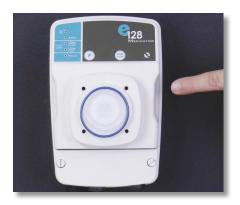
**Step 9:** If the blue o-ring is not there, still discard the pump head, but check to see if the blue o-ring is stuck to the **e128** Pump.
