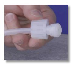
**Step 8:** Pull the tube nut toward the nozzle to compress the collar and nozzle tight together, forming a ferrule connection.
