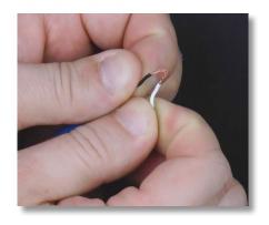
**Step 3:** Touch the e128 lead wires together to verify if the interface works.
