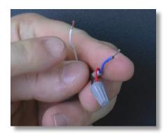
**NOTE:** Polarity typically does not matter, but if it does, the **e128** white wire is positive. Use wire nuts if necessary.
