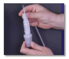
**Step 2:** Loosen the foot filter tube nut and disconnect the PVC suction tubing, tube nut, collar, and nozzle attached.
