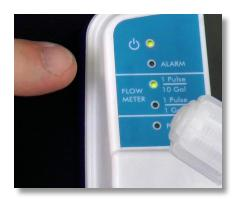
**Step 8:** Switch programs by putting the pump in standby mode and press the '**F**' or **Function** button.
