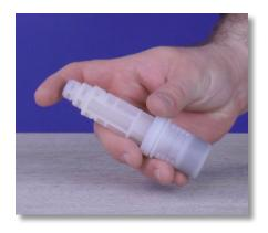
**Step 3:** Shake the foot filter back and forth. You should hear a ceramic ball moving freely inside. If not, separate the foot filter into three (3) pieces by popping the filter basket from the filter body.
