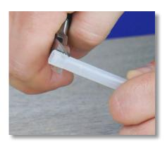
**Step 5:** Inspect the tube's condition. If the tube is cracked or looks really old, replace it now.
