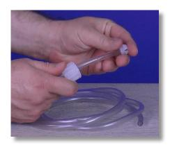
**Step 16:** Slide the collar back onto the tube, and make sure the collar's crown is pointing away from the tube nut.
