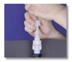
**Step 22:** Loosen the injection valve tube nut and disconnect the discharge tubing along with the tube nut, collar, and nozzle attached.
