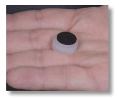
**Step 12:** Check to see if the black transit washer is stuck to the nozzle and remove.
