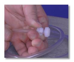
**Step 20:** If the tube nut is not securing recheck the ferrule connection. Pull the tube nut toward the nozzle, once more, to compress the collar and nozzle together. Retighten the tube nut until secure.
