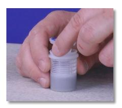
**Step 6:** Pull the filter seat out of the filter basket and set the filter basket aside.
