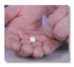
**Step 7:** Pour the ceramic ball out of the filter seat and into your hand. Set the filter seat down and use the small towel to wipe the ceramic ball clean. Do not misplace it.
