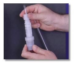
**Step 18:** Grab the foot filter and reattach the tube, and tube connections onto the foot filter by hand tightening the tube nut. Do not cross thread nor overtighten.
