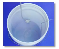
**Step 19:** Place the foot filter back into the chemical bucket or stock tank, making sure it is sitting vertically.
