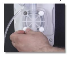
**Step 1:** Over time the pump head may work itself loose from the pump. To check this, remove the four white caps on the pump head.
