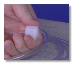
**Step 18:** Pull the tube nut toward the nozzle to compress the collar and nozzle tight together. This should form a ferrule connection.
