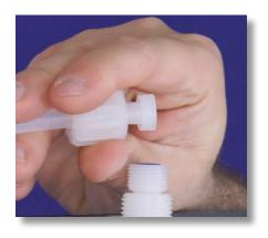
**Step 27:** Pull the tube nut toward the nozzle to compress the collar and nozzle tight together. This should form a ferrule connection.
