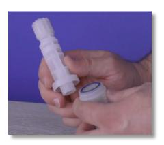
**Step 4:** The filter seat may stick to the filter body. Make sure it rests in the filter basket instead, to avoid losing the ceramic ball.
