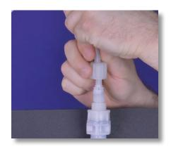
**Step 28:** Reattach the tube, and tube connections onto the injection valve by hand tightening the tube nut. Do not cross thread nor overtighten.
