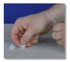
**Step 13:** Grab the PVC suction tubing hanging down from the suction valve. Remove the nozzle and collar from the tube and set aside. Do not lose them.
