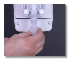
**Step 19:** Reattach the tube, and tube connections onto the suction valve by hand tightening the tube nut. Do not cross thread nor overtighten.
