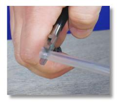
**Step 15:** Inspect the tube's condition. If the tube is cracked, rigid, or looks really old replace it now.
