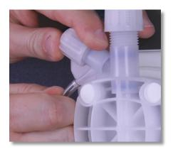
**Step 6:** Slide the bleed-off tubing back onto the air bleed barb, and place the open end of the tubing into the stock tank.
