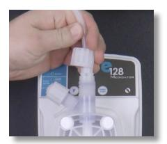
**Step 9:** Reattach the tube, and tube connections onto the discharge valve by hand tightening the tube nut. Do not cross thread nor overtighten.
