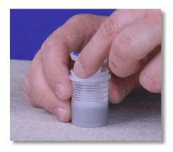
**Step 11:** Set the filter body down, grab the filter basket and put the filter seat back into the filter basket.
