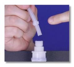
**Step 25:** Slide the collar back onto the tube, and make sure the collar's crown is pointing away from the tube nut.
