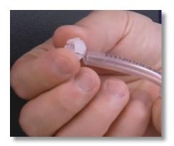
**Step 15:** Slide the collar back onto the tube, and make sure the collar's crown is pointing away from the tube nut.
