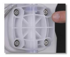
**Step 2:** Underneath the white caps are four screws. Using the Allen Wrench, tighten the four (4) screws about 1/8 turn each. Reinsert the four white caps back over the screws.
