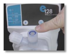
**Step 3:** Make sure not to lose the o-ring directly below the transit washer.
