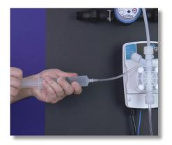
**Step 3:** Using the syringe kit, slide the syringe onto the air bleed barb and draw the plunger back. Chemistry should enter the syringe.
