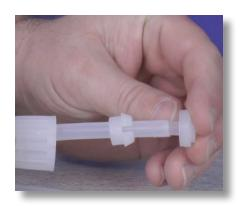
**Step 7:** Slide the nozzle back into the tube's opening. Push the collar and nozzle together as close as possible.
