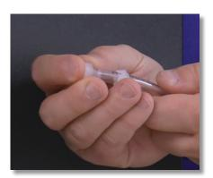
**Step 16:** Slide the nozzle back into the tube's opening. Push the collar and nozzle together as close as possible. Pull the tube nut toward the nozzle to compress the collar and nozzle tight together. This should form a ferrule connection.
