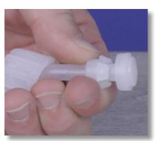
**Step 29:** If the tube nut is not securing, recheck the ferrule connection. Pull the tube nut toward the nozzle, once more, to compress the collar and nozzle together. Retighten the tube nut until secure.
