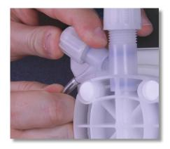
**Step 2:** Remove the bleed-off tubing from the air bleed barb and set aside.
