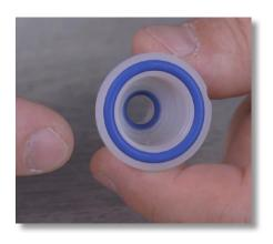
**Step 8:** While holding onto the ceramic ball, inspect the two blue o-rings in the grooves of the filter seat and make sure they are not damaged.
