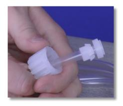
**Step 17:** Always be mindful of the orientation for the tubing connections.
