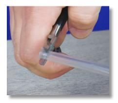
**Step 14:** Inspect the tube's condition. If the tube is cracked, rigid, or looks really old replace it now.
