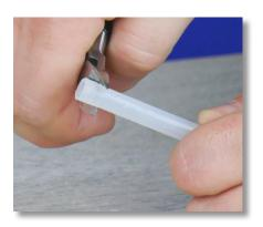
**Step 24:** Look at the end of the tube. If the tube's end is flared, use the diagonal pliers to cut the flared portion off.
