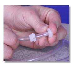
**Step 17:** Slide the nozzle back into the tube's opening. Push the collar and nozzle together as close as possible.
