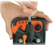
Hand tighten the discharge valve nut.
