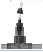
Insert the injection stem into the water line as shown below. Use Teflon tape on both threaded connections.
