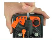
Hand tighten the discharge valve nut.
