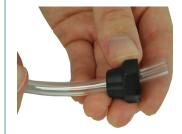
Install the suction tube onto the barb, push all the way to the threads.
