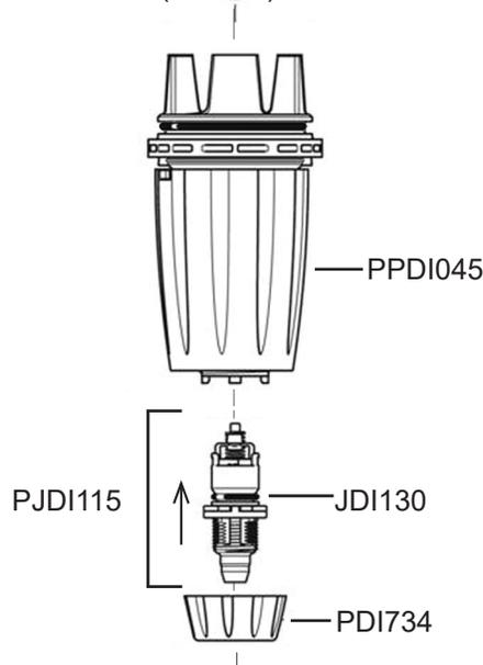
11. Lubricate the large o-ring (JDI100) on top of the injection stem assembly (PPDI045), with a small amount of **Dosa-Lube**. Insert the injection stem assembly back into the bottom of the blue body and screw back the the stem assembly nut (PDI702).
