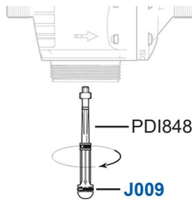
4. Remove the isolation body (PDI846) by pulling on it and place it in the solution.
