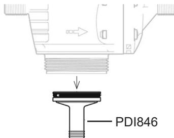
5. Unscrew the check valve nut (PDI734) and remove the check valve assembly (PJDI115), from the injection stem assembly (PPDI045), by pulling it down.
