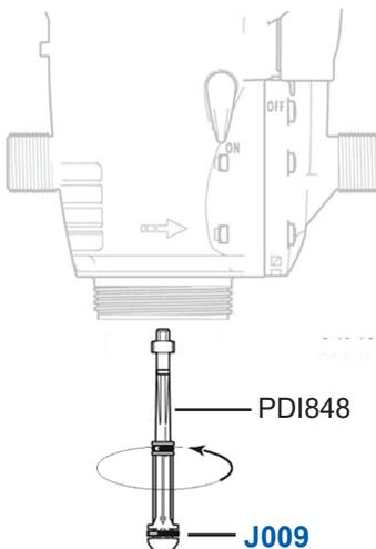
**NOTE:** Do not apply **Dosa-Lube** to the plunger seal (**J009**).
