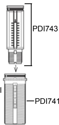
11. Slide the injection stem assembly nut (PDI702) onto the black sleeve (PDI741). Then screw the adjusting sleeve (PPDI037) back onto the black injection sleeve (PDI741).
