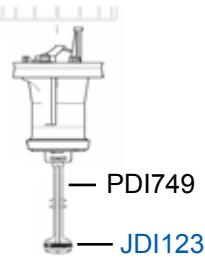
16. Insert the Piston Assembly into the lower housing (PPDI033), then screw the upper bell housing (MPDI186) back in place.
