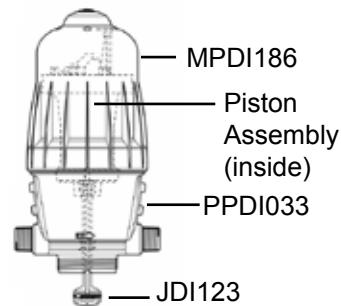
17. Attach the injection stem assembly (CDDI076) to the bottom of unit making sure the teeth on the sleeve fit into the grooves of the blue body. Screw the injection stem nut (PDI702) back on.
