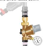
7 Connect the Tee to the other end of the Pressure Regulator assembly.
