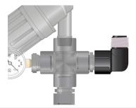
Attach the Check Valve to the Elbow, make sure the arrow points up.
