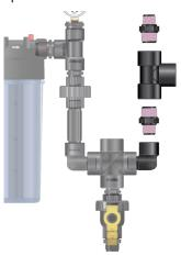
Connect the 3/4" Tee, a Close Nipple, the Check Valve (make sure arrow points down), and the Barb
