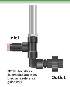
Wrap 5 to 6 turns of **Teflon**® **tape** on all threads. Make sure to wrap tape clockwise to prevent from unravelling.
