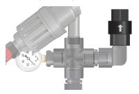
Attach the last **Nipple** to the **Elbow**.
