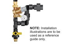
Wrap 5 to 6 turns of **Teflon® tape** on all threads.
