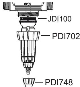
Cut 1" from the tip of the hose in a straight line. Insert the hose back onto the bottom of the check valve barb. Screw hose nut (PDI748) back on.
