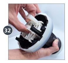
Now, test the piston assembly by carefully pulling the Push Rod up until you hear a click, then snap the last 3 Valves back on.
