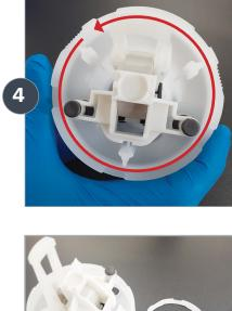
Squeeze the Locking Ring from grip points outside-edge and turn it counterclockwise to unlock the tooth.
