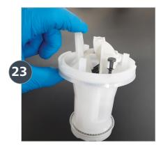
To test the piston, pull the push rod up then push down a few times, it should click in both directions.
