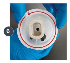
Flip the piston upside down and follow steps 3 - 4 to unlock the Lower Locking Ring.
