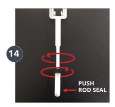
Remove Push Rod Seal by grasping and twist a quarter of a turn counterclockwise.
