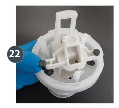
Insert the upper valves through the bottom of the top area, and snap them into the valve support frame.
