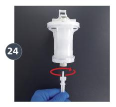
Reinstall the plunger into the bottom of the piston shell and twist a quarter turn clockwise to lock into place.
