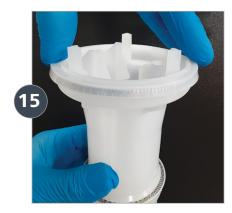
Install the NEW **Upper Piston Flange** (**MPDI243U**), with the larger end facing down, by carefully pressing it onto the upper flange mounting area as far as it goes.
