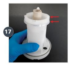
Flip the piston shell over and repeat step 15 - 16 to install the NEW Lower Piston Flange (MPDI244U) and Lower Locking Ring (PDI1237).
