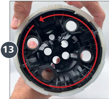
Rotate the white lock ring about  $\frac{3}{4}$  of an inch counterclockwise to unlock, making sure the white tooth slides above the black lever.
