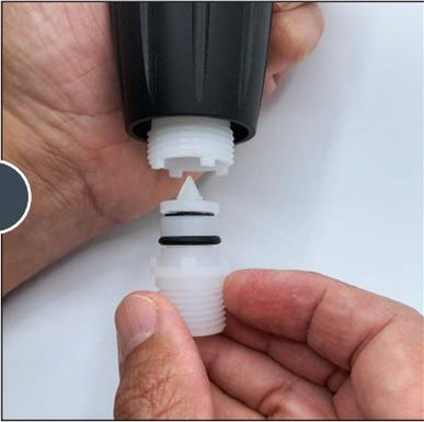
Grasp the white threaded barb and pull the Check Valve assembly straight out.
