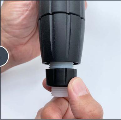
Unscrew and remove the check valve nut.
