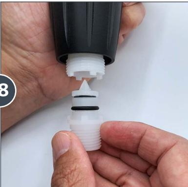
Install the new **Check Valve Assembly (Part #: PJD1215)** into the stem.
