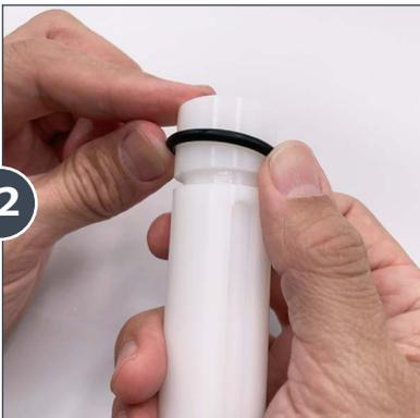
Before placing the insert back into the injection stem, remove and replace the **Injection Stem O-Ring (Part #: JDI120)**.
