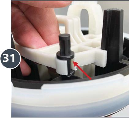
Snap one of the upper valves into the valve guide.
