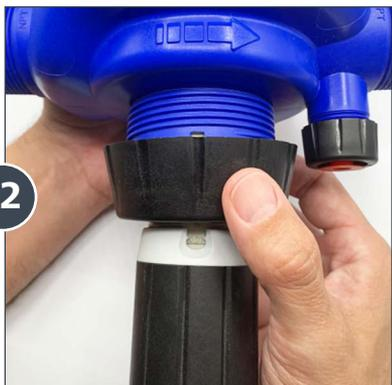
Reinstall the injection stem nut hand tight.
