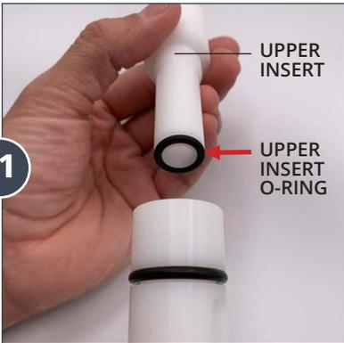
Unscrew the upper insert from the top of the injection stem, then flip the injection stem upside down so the Upper Insert O-ring comes off.
