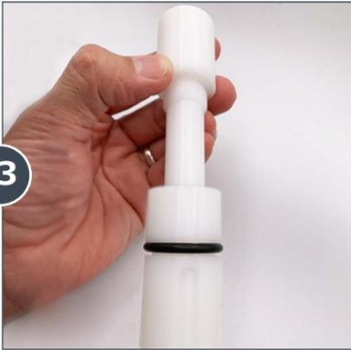
Screw the upper insert back into the top of the injection stem.
