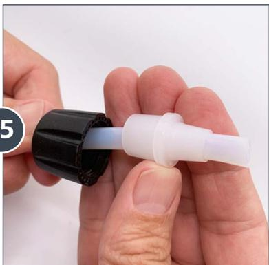
Thread the suction hose nut and ferrule onto the hose.
