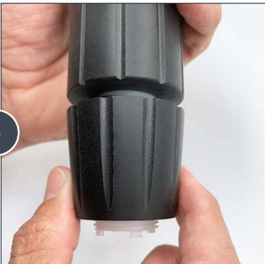
Unscrew and remove the lock nut.
