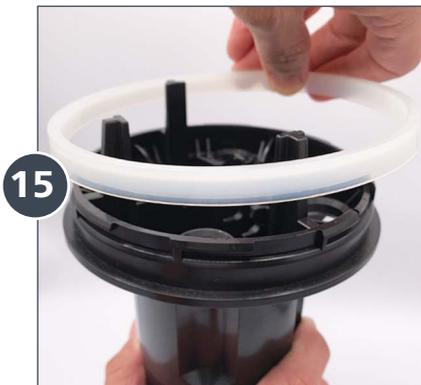
Pick up the **NEW Upper Flange (PDI1093)** and slide it onto the piston shell with the **V** shape opening facing downward, and flat edge facing up. Push down until it sits on the ledge of the black piston shell.
