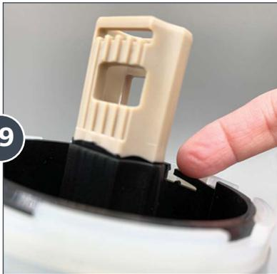
Press down on the lock lever directly next to the tooth.
