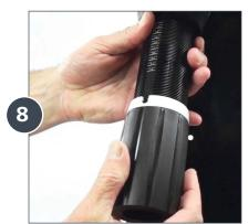
Unscrew and remove the adjusting nut.
