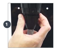
Unscrew the suction hose nut and remove the suction hose.
