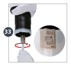
Insert the plunger back into the piston and rotate it a quarter of a turn clockwise to lock it into place.
