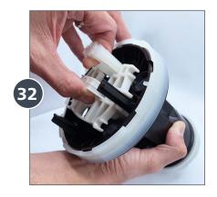
Now, test the piston assembly by carefully pulling the push rod up until you hear a click, then snap the last 3 Valves back on.
