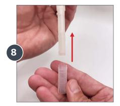
Slide the NEW **Push Rod Seal** (**PDI1085**) onto the push rod with the tapered end on the push rod. When in position, rotate the Push Rod Seal a quarter turn clockwise to lock into place.
