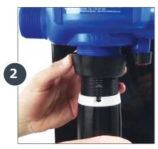
Unscrew the injection stem nut, slide it down and set aside.
