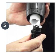
Grab the barb and pull the check valve assembly straight out and discard.
