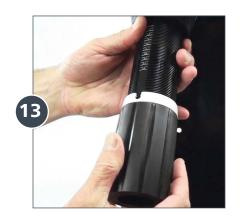
Thread the adjusting nut back onto the black injection sleeve.
