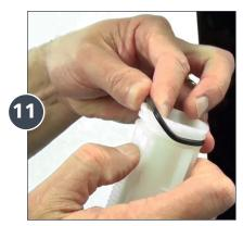
Remove and replace the **Injection Stem O-Ring** (Part #: JDI122).
