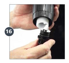
Install the new Check Valve Assembly (Part #: PJDI118) into the stem.
