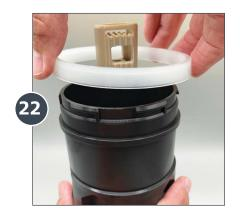
Pick up the NEW Lower Flange (PDI1092) and slide it onto the piston shell, with the V shape opening facing downward and flat edge facing up. Push down until it sits on the edge of the black piston shell.
