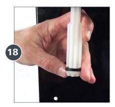
Set the stem aside and pick up the blue body. Remove the Plunger Seal by pinching and rolling it off the plunger.
