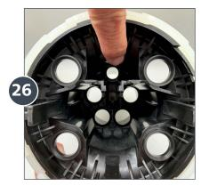
There is also a single smaller hole for the push rod assembly.
