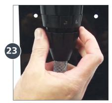
Thread the suction hose nut onto the hose. Slide the hose onto the barb. Reattach the hose nut.
