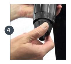
Unscrew and remove the check valve nut.
