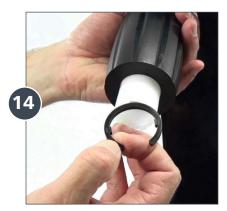
Replace the **C** clamp by sliding it over the threads. Rotate until it clicks into place.
