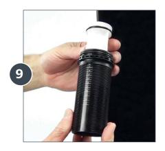
Push the white injection stem up and out of the black injection sleeve.
