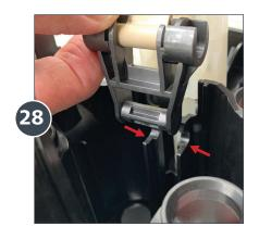
Make sure the Connecting Rod drops into the notches inside the piston shell.
