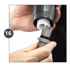
Install the new Check Valve Assembly (Part #: PJDI232) into the stem.
