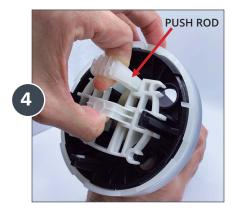
Raise the push rod carefully and pull the piston's mechanism up and out of black piston shell.
