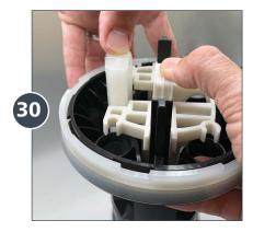
Carefully begin pressing the mechanism (both assemblies) into place inside the piston shell and double check the alignment of both sections.
