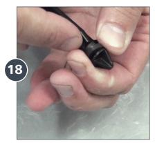
Set the stem aside and pick up the blue body. Remove the Plunger Seal by pinching and rolling it off the plunger.
