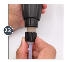
Thread the suction hose nut onto the hose. Slide the hose onto the barb. Reattach the hose nut.
