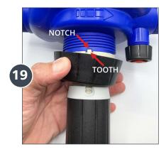
Insert the plunger inside the top of the stem in a vertical motion to avoid bending the plunger.
