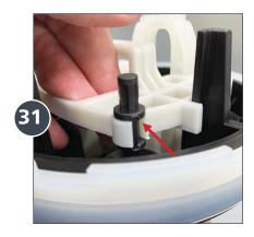
Snap one of the upper valves into the valve guide.
