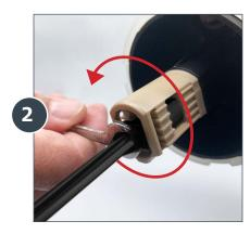
Remove the plunger from the piston by rotating it a quarter of a turn counterclockwise.
