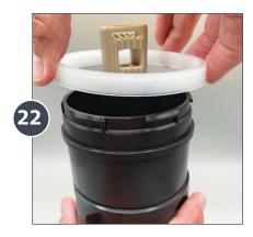
Pick up the NEW **Lower Flange** (**PDI1092**) and slide it onto the piston shell, with the **V** shape opening facing downward and flat edge facing up. Push down until it sits on the edge of the black piston shell.
