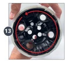
Rotate the white lock ring about <sup>3</sup>/<sub>4</sub> of an inch counterclockwise to unlock, making sure the white tooth slides above the black lever.
