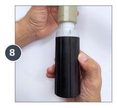
Unscrew and remove the adjusting nut.
