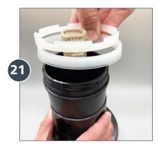
Slide the lock ring and Lower Flange up and off the black piston shell.
