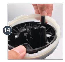
Slide the white lock ring and Upper Flange up and off the black piston shell.
