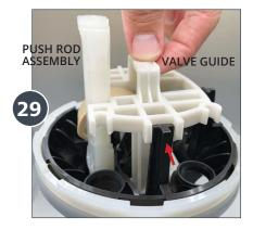
Align the valve rack next to the push rod assembly making sure the guide aligns with the black posts on the piston shell, and the lower valves align with the 4 center openings.
