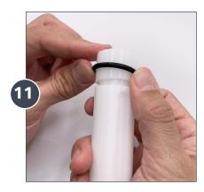
Remove and replace the **Injection Stem O-Ring** (Part #: JDI120).
