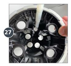
Insert the push rod assembly inside the smaller hole with the top curved portion facing outward (following the curve of the piston).
