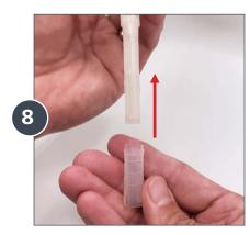
Slide the NEW **Push Rod Seal** (**PDI1085**) onto the push rod with the tapered end on the push rod. When in position, rotate the Push Rod Seal a quarter turn clockwise to lock into place.
