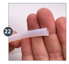
Before installing the suction hose, inspect it. If it flares out, cut an inch or so off and reinstall.
