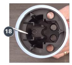
Before reinstalling the push rod and valve support assembly, look inside the piston shell. You will notice four holes in a line and a single hole on the other side.
