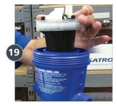
Carefully press the piston back into the injector and install the bell housing.
