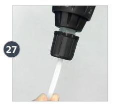
After you tighten the nut, pull on the hose to make sure it is connected securely.
