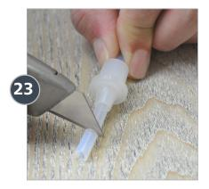
Before installing the suction hose, slide the ferrule back onto the hose. Cut a half inch off the top of the hose.
