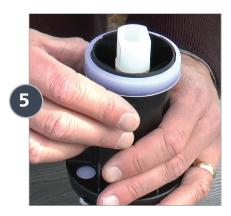
Flip the piston upside down and follow steps 3 and 4 to remove the lower or smaller diameter flange.
