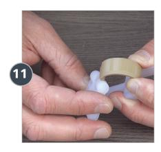
Slide the other end of the Omega spring into the new **Connecting Rod** (Part #: **PDI649**). The key to this step is to make sure the curved top of the push rod faces in the same direction as the Omega spring.
