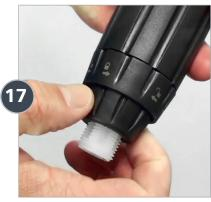
Reinstall the check valve nut.
