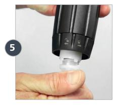
Grab the barb and pull the check valve assembly straight out. It usually comes out in two pieces. Discard all check valve parts.
