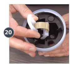
To demonstrate the alignment of the push rod assembly, the curved top would face inward, inserting the push rod into the single hole. This is where the connecting rod sits in the piston.
