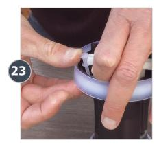
Insert the upper valves into the bottom of the upper area, snapping them into the valve support frame.
