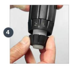
Unscrew and remove the check valve nut.
