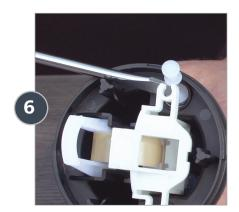
To remove the motor and valve support assembly from the piston shell, you will need a flat head screwdriver. Using the screwdriver, remove the upper valves from the guide. The valves look like golf tees and will drop down and out of the piston shell. Set them aside.
