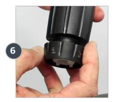
Unscrew and remove the lock nut.
