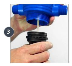
Pull the injection stem straight out from the body of the injector. Set the nut and body aside.
