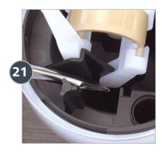
The key is to make sure the white connecting rod drops into the notches inside the piston shell.
