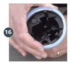
Align the tooth with the shell and press down and twist a quarter turn clockwise to lock. If it is difficult to twist or if the flange lifts up easily, just remove the flange, realign and try again.
