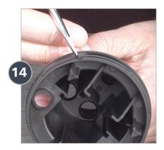
Now locate the notch on the piston shell.
