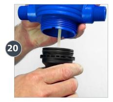
To finish up, carefully insert the plunger into injection stem assembly.
