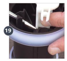
Notice how the valve support frame aligns on the side with the four holes, making sure it goes into the grooves.
