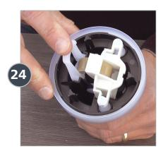
To test the piston pull the push rod up and press it down a few times. It should click in both directions.
