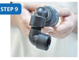
Attach the other **street elbow** to the end of the elbow and turn to a  $90^{\circ}$  angle, as shown.
