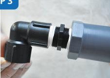
Thread the **3/4**" female to female elbow to the nipple and hand tighten.
