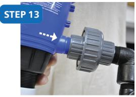
Pick up the **outlet assembly** and attach the **union** to the outlet side of the Dosatron. Note the direction of the arrow. Hand tighten.
