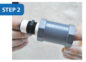
To assemble the inlet side, hold the **flow restrictor** in one hand and attach a **2" nipple** to the other side.
