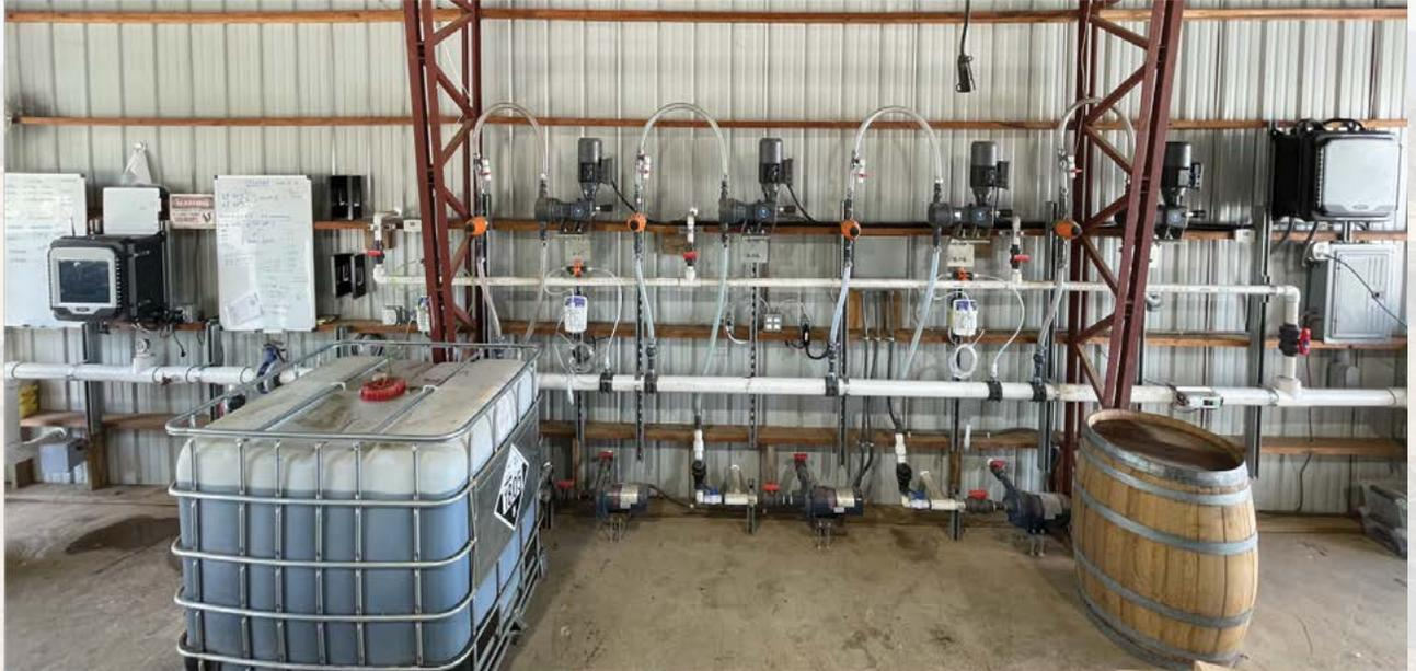
The in-line, Direct Inject, Mega-Flow System blends recipes on demand so that waste of costly inputs is minimized. Detailed Reporting delivers information including total application rates, per input, for every scheduled event.
