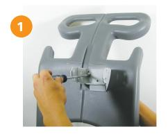
Install the mounting bracket, included with your Dosatron pump, to the Li'l Bud-D cart using the hardware kit provided.
