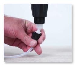
**Step 4:** Insert the hose back into the barb and hand tighten the nut.
