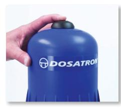
**Step 6:** Press the air bleed button on the bell housing a few times to release the pressure.
