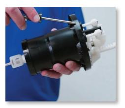
**Step 5:** Next, visually inspect the upper and lower flanges on the piston shell. If they are worn or have deep scratches, the piston shell (Part #: 8PC002) needs to be replaced.
