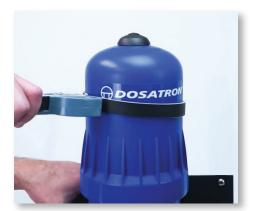
**Step 2:** Use the strap wrench (Part #: TOOL01) to loosen the bell housing. Unscrew, remove and set it aside.
