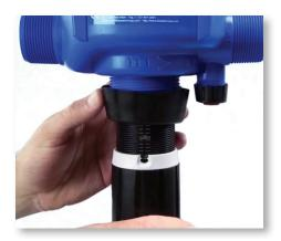
Step 8: Unscrew the injection stem nut and remove.
