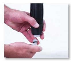
**Step 3:** Grasp the white threaded barb and pull the check valve assembly straight out. It might come out in two pieces. Set the unit aside.
