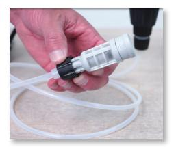
If your Dosatron is clicking but not drawing the concentrate, it could be as simple as the strainer is plugged with debris.
