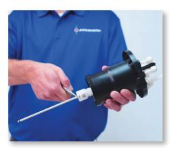
**Step 6:** If you removed the plunger in the last step, reattach now using the needle nose pliers, by aligning the top of the plunger with the retainer. Twist the plunger clockwise to lock.
