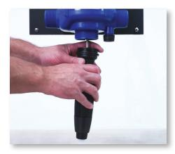
**Step 9:** Then, pull the injection stem straight out of the injector's body and set aside.
