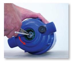
**Step 12:** Position the needle nose pliers near the top of the plunger and carefully twist it a quarter turn counter clockwise, as pictured, and disconnect.
