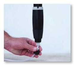
**Step 15:** Now, slide the hose into the barb and hand tighten the nut. Pull on the hose to make sure it's connected securely.
