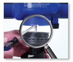
**Step 14:** Align the notches in the lower part of the blue body with the teeth on the top of the injection stem assembly. Slide the two parts together, and hand tighten the injection stem nut.
