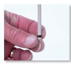
**Step 10:** Take a close look at the plunger rod and seal. Make sure the rod is straight and that the seal is free of nicks, scratches, or wear.
