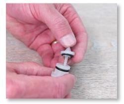
**Step 5:** To reassemble, place the new check valve assembly into the top of the barb.
