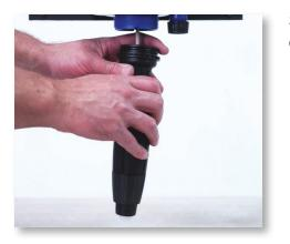
**Step 13:** Grab the injection stem assembly and carefully slide it onto the plunger as pictured.
