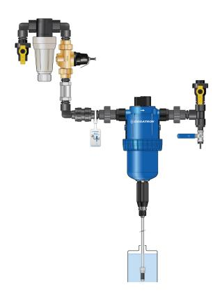
1" polypropylene single union ball valve 1/2" stainless steel ball valve 1" poly 200 mesh tee filter 1" brass pressure regulator w/gauge 1" 20 GPM flow restrictor 1" polypropylene check valve 1" unions schedule 80 PVC 1" x 2" polypropylene fittings 1/2" x 2" polypropylene fittings 1/2" x 1/2" barb fitting 1" to 3/4" reducer bushing 3/4" male to 1/2" female reducer bushing 1" Tee 1" street elbows Roll of Teflon tape Instruction card Zip tie
