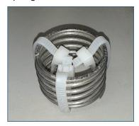
**10.** Insert the bound spring and retainer/spring connection into position as shown in photo.
