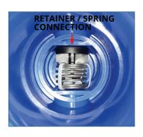
11. Carefully cut the zip ties away from spring and remove zip tie pieces. Spring will set tension when the zip ties no longer bind.
