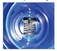
**12.** Install the bypass retainer as shown in the photo and secure the set screw.
