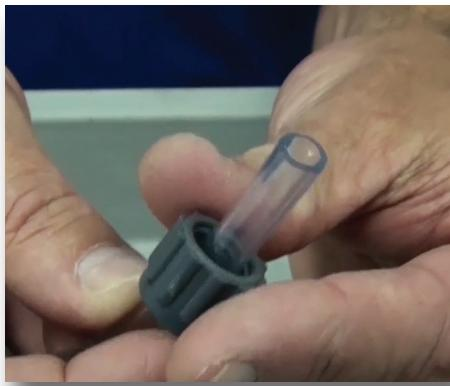
**Step 30:** Now, thread the suction hose nut onto the hose.
