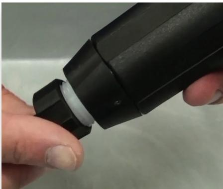
**Step 22:** Thread the barb onto the white stem and hand tighten.
