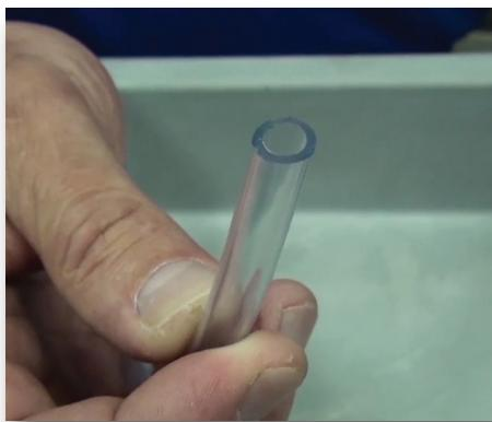
**Step 29:** Before installing the suction hose, inspect it. If it flares out, cut an inch or so off and reinstall. Or, if the suction hose is cracked, rigid, or really old, just replace it.
