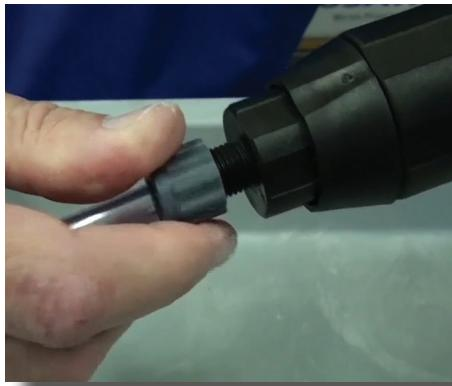
**Step 32:** Hand tighten the nut.
