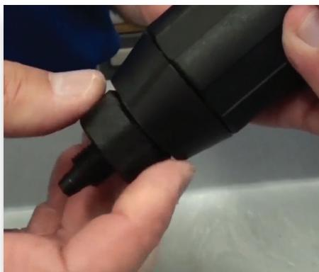
**Step 5:** Unscrew and remove the check valve (Part #: P169) barb.
