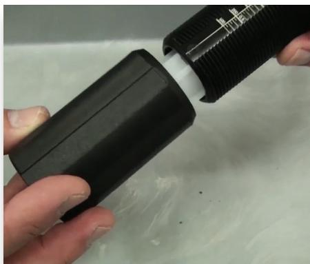
**Step 17:** Thread the adjusting nut back onto the sleeve.
