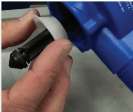
**Step 25:** If the white plastic retainer slides down, just reposition it with the slender part up into the body.
