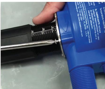
**Step 3:** Unscrew the four screws at the base of the injection stem.
