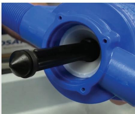
**Step 26:** The retainer should be pushed all the way up, like this.
