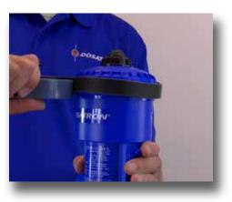
**Step 6:** Use the strap wrench to loosen the lid. Then, remove it and set aside.
