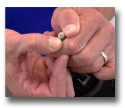
**Step 9:** To repace the seal, pinch it and roll it off of the plunger. Install the new seal into the groove.
