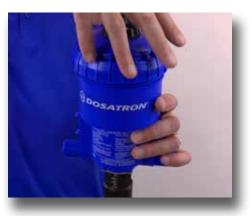
**Step 11:** Replace the lid hand tight. Slowly turn the water on and the unit should begin to click. It should be drawing the concentrate.
