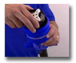
**Step 10:** Carefully insert the piston back into the body.
