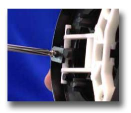
**Step 8:** To replace the piston shell, use a small tip Phillips screwdriver and remove the valve support screw.
