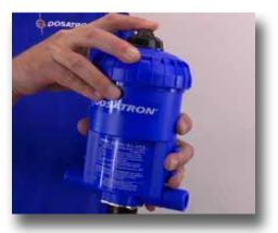
**Step 5:** To do this, turn the water off and press the air bleed button on the lid a few times to release the pressure.
