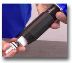
**Step 3:** Grasp the white barb and pull the check valve assembly straight out. It usually comes out in two pieces.
