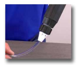
**Step 4:** If you feel suction, cut a half-inch off the top of the hose and reattach it. But, if the hose is cracked, rigid, or looks really old just replace it.
