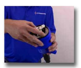
Step 20: Insert the piston back into the body.
