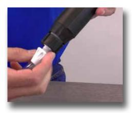
**Step 1:** It's time to investigate the check valve. To do this, remove the hose nut and hose. Set them aside.
