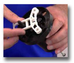
**Step 17:** Reinstall the valve support by sliding it onto the inlet valve.
