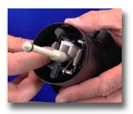
**Step 5:** Check the two actuator springs (Part #: M238) on the bottom. If they are broken or missing, just replace them.
