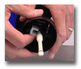
**Step 16:** Press the white plastic portion of the actuator side to side. If there is movement, re-tighten the screws.
