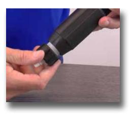
**Step 2:** Unscrew and remove the check valve nut.
