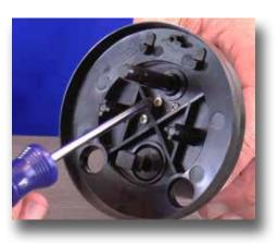
**Step 11:** Next, remove the four screws in the center of the piston shell to release the actuator assembly.
