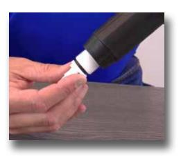
**Step 8:** Press it into the stem as shown. Hand tighten the check valve nut.
