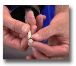
**Step 8:** Take a close look at the plunger seal (Part #: JDI106) for nicks, scratches, or wear. If you see damage, or don't remember the last time you changed the seal, just replace it now.
