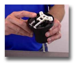
**Step 4:** Inspect the white valve support on the top and press the pushrod down.
