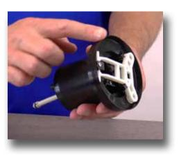
**Step 6:** You can visually inspect the upper and lower flanges on the piston shell. If they are worn or have deep scratches, the piston shell (Part #: P421) and push rod o-ring (Part #: J020) need to be replaced.
