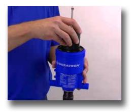
**Step 7:** Also, check the piston shell's fit inside the body. To do this, invert the piston and slide it into the body. It should be a snug fit. If it feels loose, the piston shell (Part #: P421) and push rod o-ring (Part #: J020) need to be replaced.
