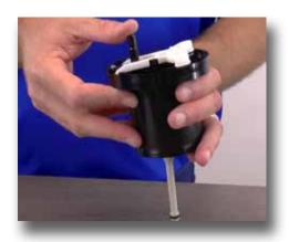
**Step 19:** Test the piston, by pressing the pushrod from the top and bottom, it should click each time.
