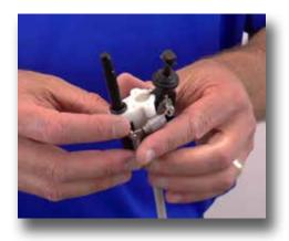
**Step 13:** Put the new push rod o-ring on top of the push rod and slide it down as far as it will go.
