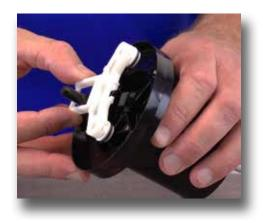
**Step 10:** Press the pushrod up and slide the valve support off the inlet valve and set aside.
