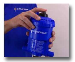
**Step 1:** Turn the water off and press the air bleed button on the top of the lid a few times to release the pressure.
