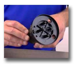
**Step 14:** Position the actuator assembly in the shell as shown and hold firmly.
