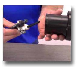
**Step 12:** Pull the actuator assembly out and discard the old piston shell.
