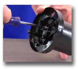
**Step 15:** Now re-install the four screws and hand-tighten them in a star pattern.
