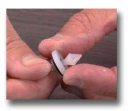
**Step 5:** To investigate the check valve, carefully lift the cone from the retainer. Look at the bottom side of the cone.
