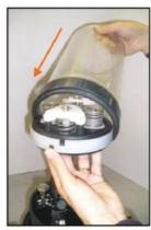
With piston ring in place, hold piston assembly in one hand at the compression point and with other hand hold on to the glass tube from the top. Make sure to insert the glass in the direction of the axis created by the two white flapper valves (see picture). Approach the piston head with the glass tube at a 45-degree angle. Do not force glass over piston assembly. Be patient, back off if needed, re-lubricate the glass and try again.
