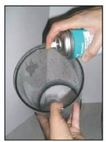
Clean and lubricate the inside lower half of the glass tube with soapy water or silicone spray to ease reinstallation.
