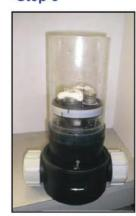
Place the glass tube on the black base, and secure it using the wire.
