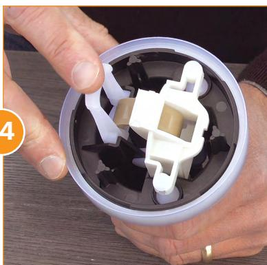
To test the piston pull the push rod up and press it down a few times. It should click in both directions.
