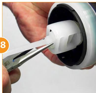
Reinstall the **Plunger with Seal** (Part #: PJDI138) into the bottom of the piston shell. Using the needle nose pliers twist the plunger a quarter turn clockwise to lock.
