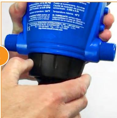
Unscrew the injection stem nut.
