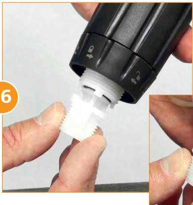
Install the new **Check Valve Assembly** (Part #: PJDI140) into the stem. Make sure it is in the position shown before inserting into the stem.
