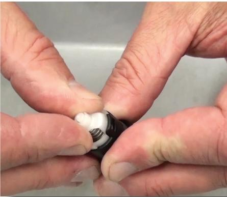
**Step 11:** Align the guide and twist it 1/4 turn clockwise to lock. Give it a tug to make sure everything is in position.
