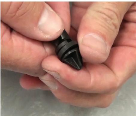
**Step 14:** Set the stem aside and pick up the blue body. Remove the plunger seal (Part #: J009) by pinching it and rolling it off the plunger.
