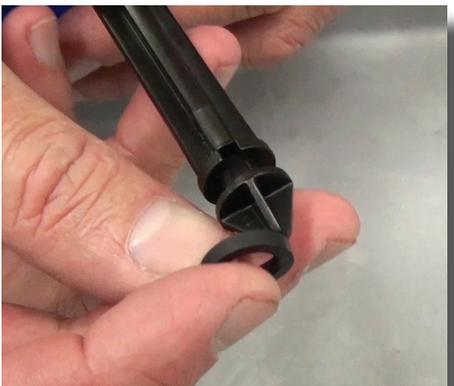
**Step 15:** Install the new seal onto the groove on the plunger.
