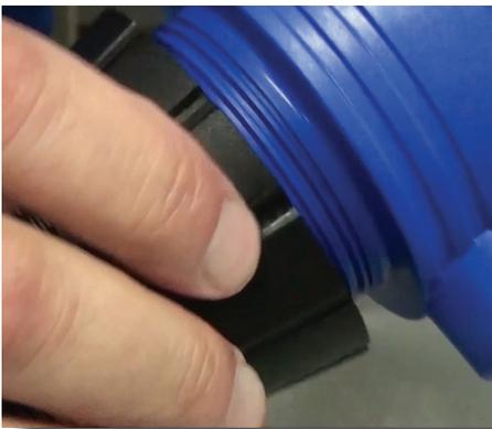
**Step 17:** Reinstall the injection stem nut, hand tight.
