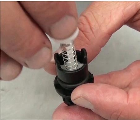
**Step 10:** Slide the new spring over the shaft and position the new top guide over the shaft.
