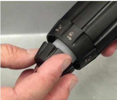
**Step 13:** Reinstall the check valve nut.
