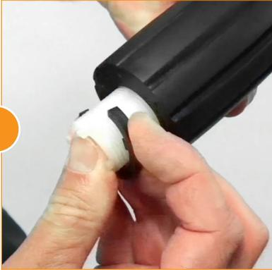
Remove the C clamp by spreading the opening and sliding it down over the threads.
