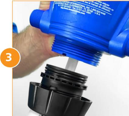
Pull the injection stem straight out from the body of the injector. Set the body aside.
