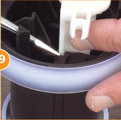
Notice how the valve support frame aligns on the side with the four holes, making sure it goes into the grooves.
