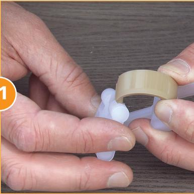
Slide the other end of the Omega spring into the new **Connecting Rod (Part #: PDI649)**. The key to this step is to make sure the curved top of the push rod faces in the same direction as the Omega spring.
