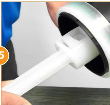
Reinstall the plunger into the bottom of the piston shell and twist a quarter turn clockwise to lock.
