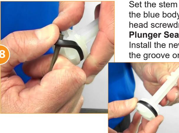
Set the stem aside and pick up the blue body. Using a small flat head screwdriver, remove the **Plunger Seal (Part #: JDI123)**. Install the new plunger seal into the groove on the plunger.
