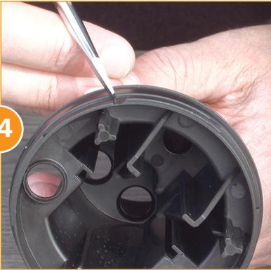
Now locate the notch on the piston shell.
