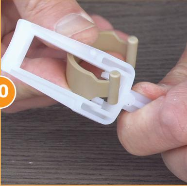
Twist to remove the Omega spring out of the push rod.
