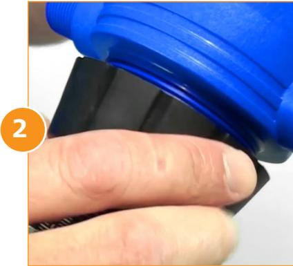
Unscrew the injection stem nut.
