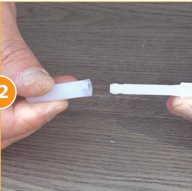
Replace the **Push Rod Seal (Part #: PDI648)**. Remove by grasping and turning counter clockwise. Carefully slide the new push rod seal onto the push rod as far as it will go and twist a quarter turn clockwise to lock.
