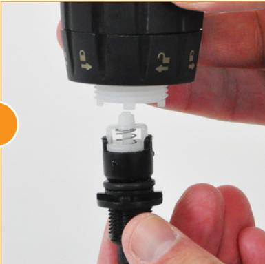
Grab the barb and pull the check valve assembly straight out and discard.
