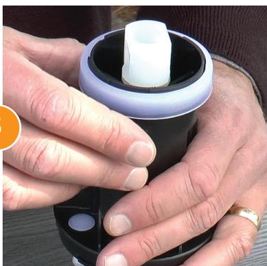
Flip the piston upside down and follow steps 3 and 4 to remove the lower or smaller diameter flange.
