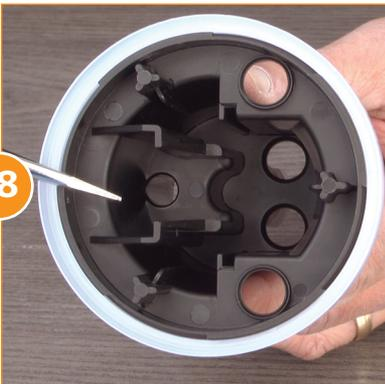
Before reinstalling the push rod and valve support assembly, look inside the piston shell. You will notice four holes in a line and a single hole on the other side.
