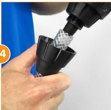
Thread the suction hose nut onto the hose. Slide the hose onto the barb. Reattach the hose nut.
