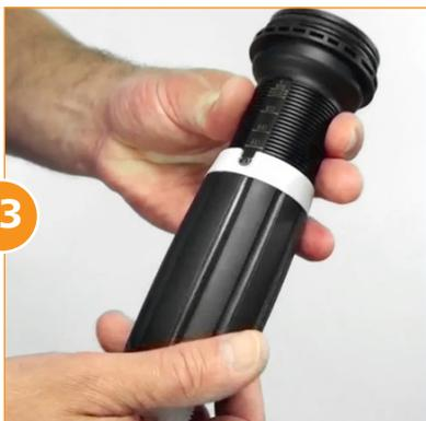
Slide the injection stem nut up onto the sleeve, and thread the adjusting nut back on.
