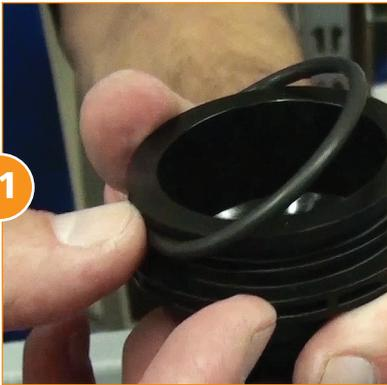
Remove and replace the **Sleeve O-Ring (Part #: JDI100)**.
