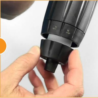
Unscrew and remove the check valve nut.
