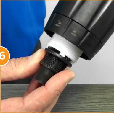
Install the new **Check Valve Assembly** into the stem.
