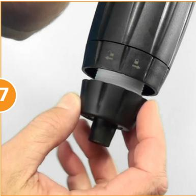
Reinstall the check valve nut.
