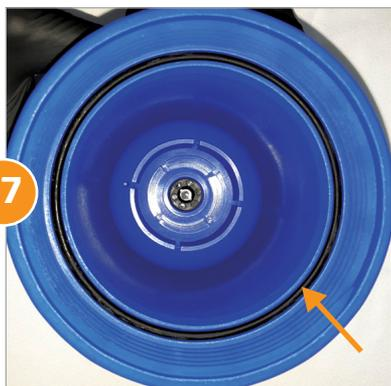
Hold the bell housing. Remove and discard the bell housing o-ring.
