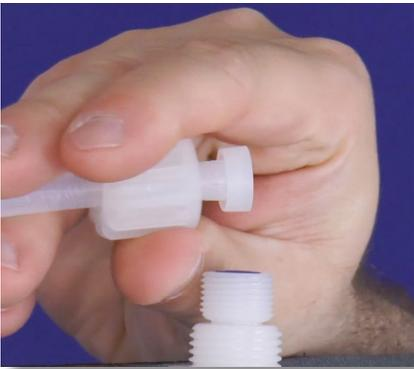
**Step 99:** Slide the nozzle back into the tube's opening. Push the collar and nozzle together as close as possible.
