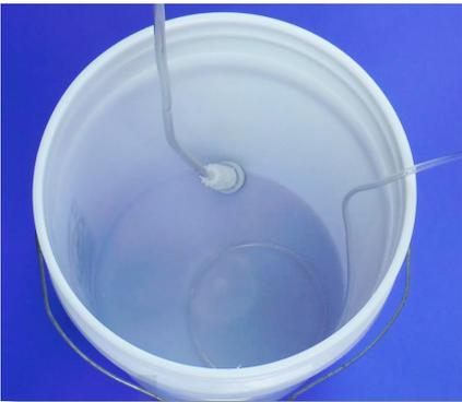
**Step 62:** Inspect the foot filter by taking it out of the chemical bucket or stock tank.
