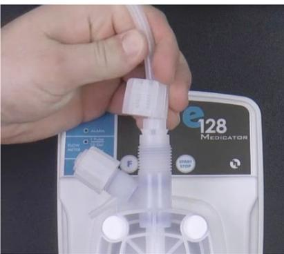
**Step 141:** Reattach the tube, and tube connections onto the discharge valve by hand tightening the tube nut. Do not cross thread nor overtighten.
