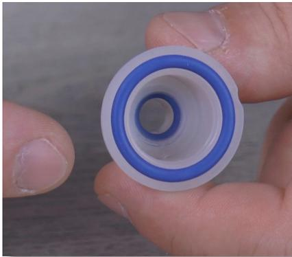
**Step 69:** While holding onto the ceramic ball, inspect the two blue o-rings in the grooves of the filter seat and make sure they are not damaged.
