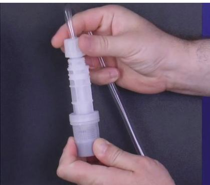
**Step 79:** Grab the foot filter and reattach the tube, and tube connections onto the foot filter by hand tightening the tube nut. Do not cross thread nor overtighten.
