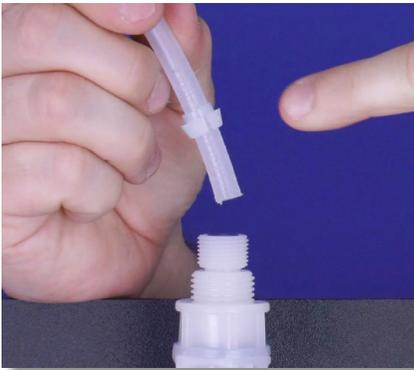
**Step 146:** Slide the collar back onto the tube, and make sure the collar's crown is pointing away from the tube nut.
