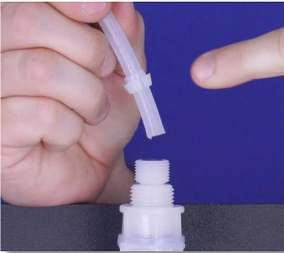
**Step 98:** Slide the collar back onto the tube, and make sure the collar's crown is pointing away from the tube nut.
