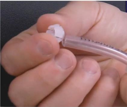
**Step 125:** Slide the collar back onto the tube, and make sure the collar's crown is pointing away from the tube nut.
