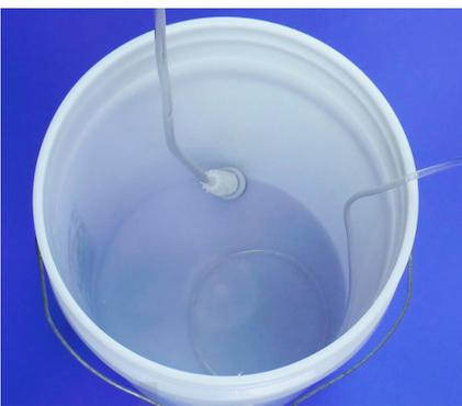
**Step 53:** Place the foot filter back into the chemical bucket or stock tank, making sure it is sitting vertically.
