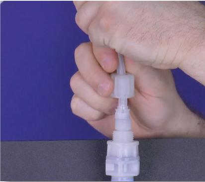
**Step 33:** Reattach the tube, and tube connections onto the injection valve by hand tightening the tube nut. Do not cross thread nor overtighten.
