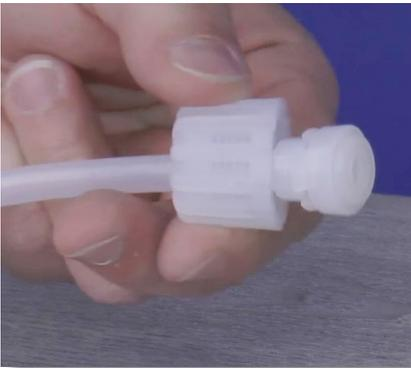
**Step 140:** Pull the tube nut toward the nozzle to compress the collar and nozzle tight together, forming a ferrule connection.
