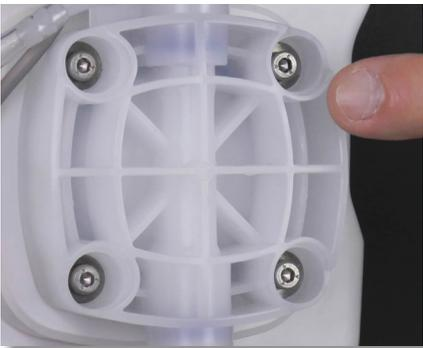
**Step 55:** Underneath the white caps are four screws. Using the Allen wrench, tighten the four (4) screws about 1/8 turn each. Reinsert the four white caps back over the screws.
