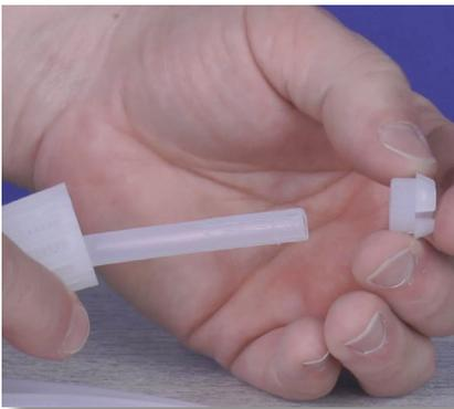
**Step 11:** Slide the collar back onto the tube, and make sure the collar's crown is pointing away from the tube nut.
