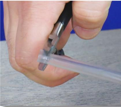
**Step 107:** . Look at the end of the tube. If the tube's end is flared, use the diagonal pliers to cut the flared portion off.
