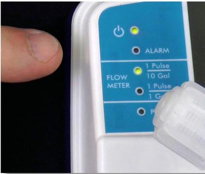
**Step 160:** Switch programs by putting the pump in standby mode and press the '**F**' or **Function** button.
