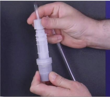
**Step 51:** Grab the foot filter and reattach the tube, and tube connections onto the foot filter by hand tightening the tube nut. Do not cross thread nor overtighten.
