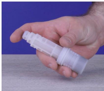
**Step 64:** Let the tubing hang from the pump head while you inspect the foot filter. Shake it back and forth. You should hear a ceramic ball moving freely inside.
