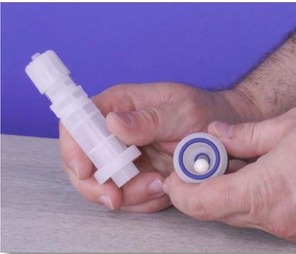
**Step 66:** Set the filter body aside and locate the ceramic ball in the filter seat.
