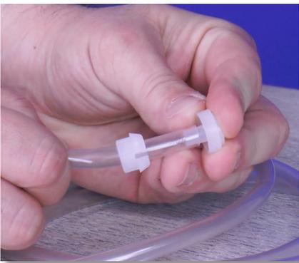
**Step 109:** Slide the nozzle back into the tube's opening. Push the collar and nozzle together as close as possible.
