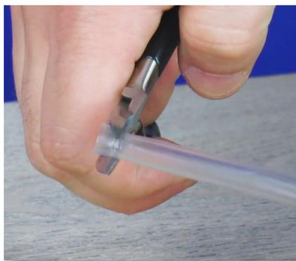
**Step 124:** Look at the end of the tube. If the tube's end is flared, use the diagonal pliers to cut the flared portion off.
