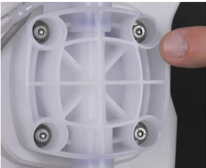
**Step 132:** Underneath the white caps are four screws. Using the Allen Wrench, tighten the four (4) screws about 1/8 turn each. Reinsert the four white caps back over the screws.
