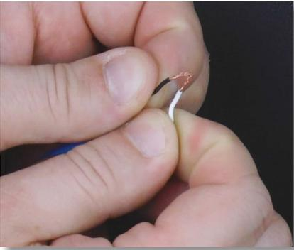
**Step 5:** Touch the e128 lead wires together to verify if the interface works.
