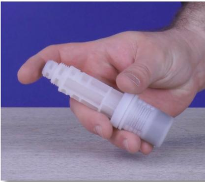
**Step 114:** Let the tubing hang from the pump head while you inspect the foot filter. Shake it back and forth. You should hear a ceramic ball moving freely inside.
