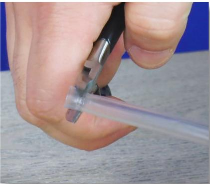
**Step 75:** Look at the end of the tube. If the tube's end is flared, use the diagonal pliers to cut the flared portion off.
