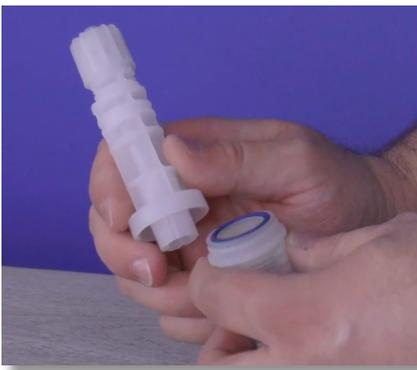
**Step 115:** If not, separate the foot filter into three (3) pieces by popping the filter basket from the filter body.
