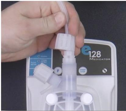
**Step 93:** Reattach the tube, and tube connections onto the discharge valve by hand tightening the tube nut. Do not cross thread nor overtighten.
