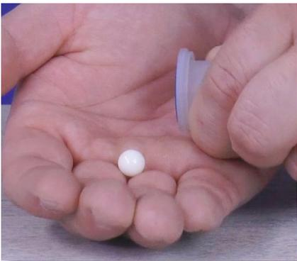
**Step 118:** Pour the ceramic ball out of the filter seat and into your hand. Set the filter seat down and use the small towel to wipe the ceramic ball clean. Do not misplace it.
