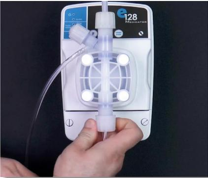
**Step 16:** locate the Suction Valve at the bottom of the Pump Head.
