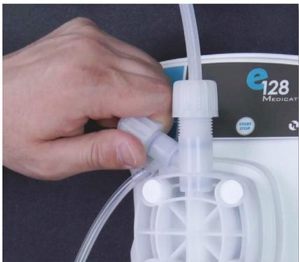
**Step 56:** Locate the air bleed valve on the upper left portion of the pump head and open it by turning the valve counter clockwise.
