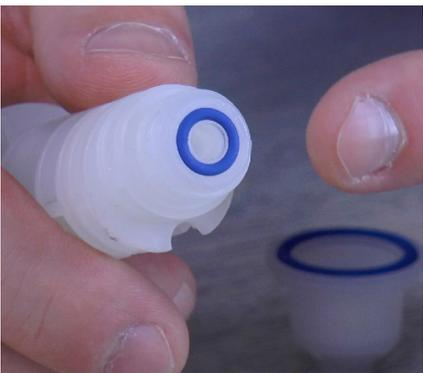
**Step 44:** Grab the filter body and inspect to make sure the small blue o-ring on the top of the filter body is not damaged.
