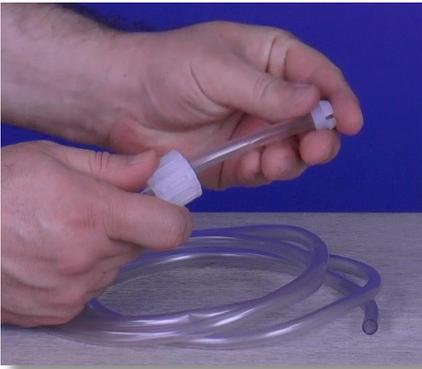
**Step 21:** Slide the collar back onto the tube, and make sure the collar's crown is pointing away from the tube nut.
