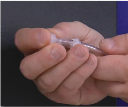
**Step 77:** Slide the nozzle back into the tube's opening. Push the collar and nozzle together as close as possible.
