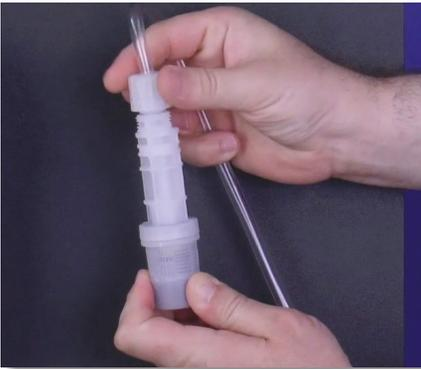
**Step 113:** Loosen the foot filter tube nut and disconnect the PVC suction tubing, tube nut, collar, and nozzle attached.
