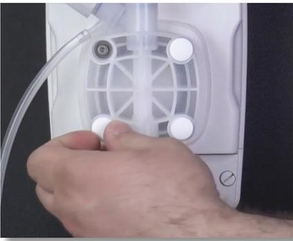
**Step 54:** Over time the pump Head may work itself loose from the pump. To check this, remove the four white caps on the pump head.
