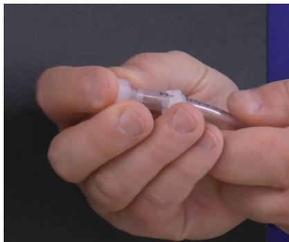
**Step 50:** Slide the nozzle back into the tube's opening. Push the collar and nozzle together as close as possible. Pull the tube nut toward the nozzle to compress the collar and nozzle tight together. This should form a ferrule connection.
