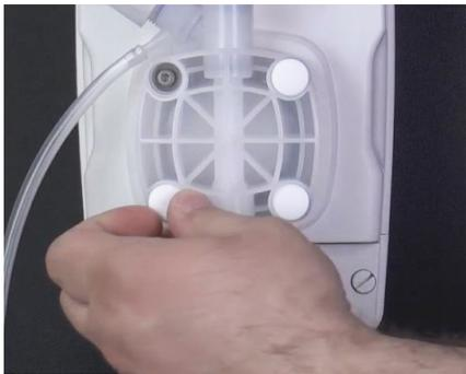
**Step 87:** Over time the pump head may work itself loose from the pump. To check this, remove the four white caps on the pump head.
