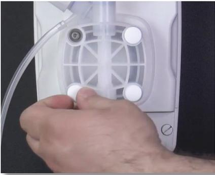
Over time the pump head may work itself loose from the pump.
