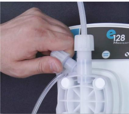
**Step 82:** Locate the air bleed valve on the upper left portion of the pump head and open it by turning the valve counter clockwise.
