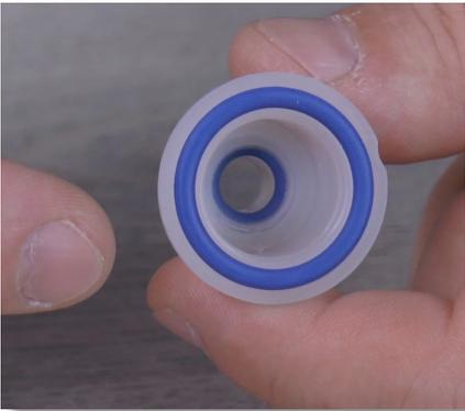
**Step 119:** While holding onto the ceramic ball, inspect the two blue o-rings in the grooves of the filter seat and make sure they are not damaged. Put the ceramic ball back into the filter seat and set the filter seat aside.
