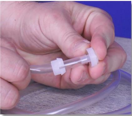
**Step 22:** Slide the nozzle back into the tube's opening. Push the collar and nozzle together as close as possible.
