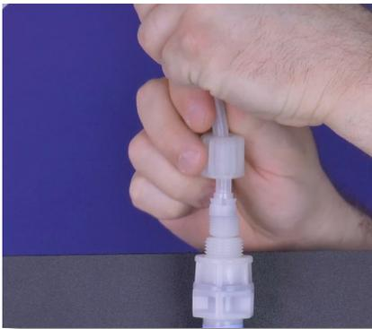
**Step 149:** Reattach the tube, and tube connections onto the injection valve by hand tightening the tube nut. Do not cross thread nor overtighten.
