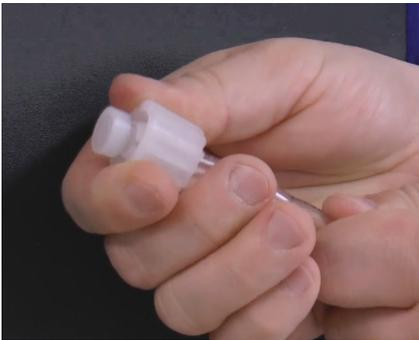
**Step 78:** Pull the tube nut toward the nozzle to compress the collar and nozzle tight together, forming a ferrule connection.
