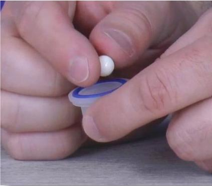
**Step 43:** Put the ceramic ball back into the filter seat and set the filter seat aside.
