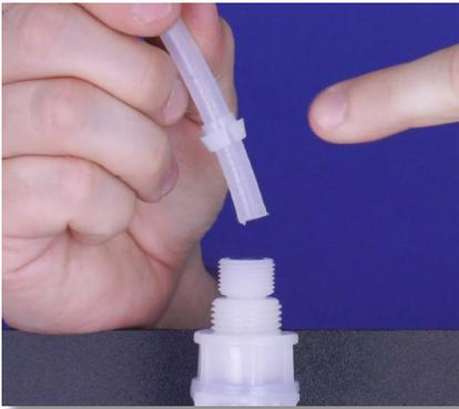
**Step 30:** Slide the collar back onto the tube, and make sure the collar's crown is pointing away from the tube nut.
