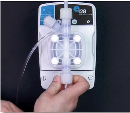
**Step 105:** . Loosen the suction valve tube nut and disconnect the PVC suction tube, tube nut, collar, and nozzle attached.
