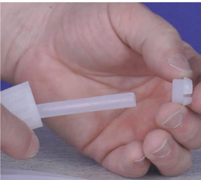
**Step 138:** Slide your collar back onto the tube, and make sure the collar's crown is pointing away from the tube nut.
