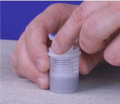
**Step 40:** Pull the filter seat out of the filter basket and set the filter basket aside.
