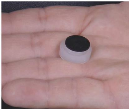
**Step 17:** Check to see if the black transit washer is stuck to the nozzle and remove.
