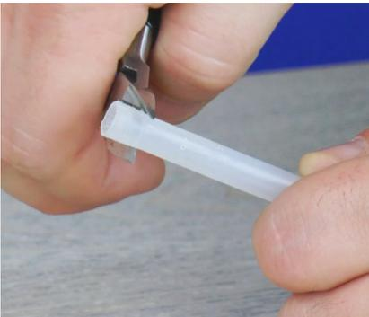
**Step 137:** Look at the end of the tube. If the tube's end is flared, use the diagonal pliers to cut the flared portion off.
