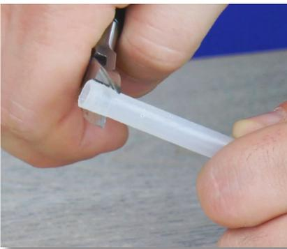
**Step 97:** Look at the end of the tube. If the tube's end is flared, use the diagonal pliers to cut the flared portion off.
