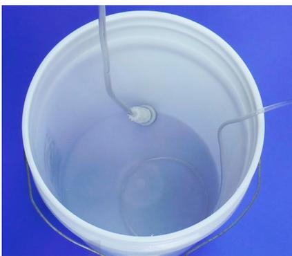
**Step 130:** To finish up, look at the PVC suction's tube condition. If the tube is cracked, rigid, or looks really old replace it now.
