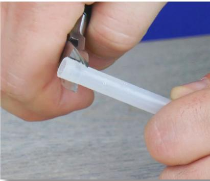
**Step 90:** Look at the end of the tube. If the tube's end is flared, use the diagonal pliers to cut the flared portion off.
