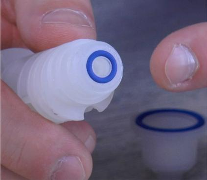
**Step 120:** Grab the filter body and inspect to make sure the small blue o-ring on the top of the filter body is not damaged.
