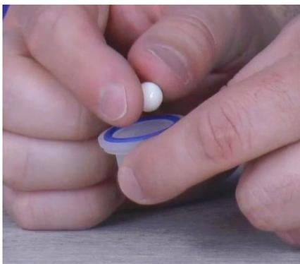
**Step 70:** Put the ceramic ball back into the filter seat and set the filter seat aside.
