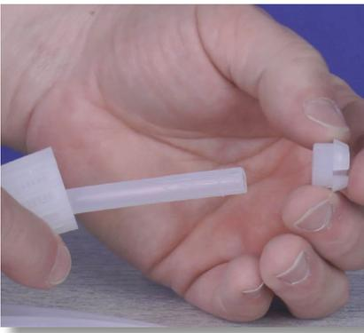
**Step 91:** Slide the collar back onto the tube, and make sure the collar's crown is pointing away from the tube nut.
