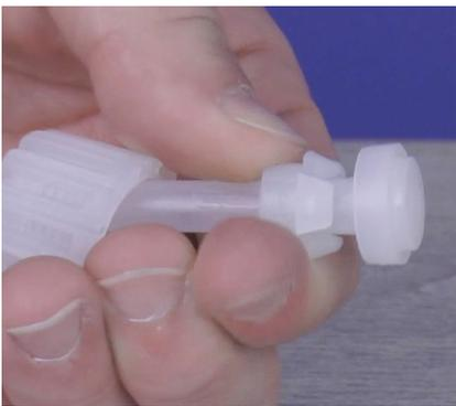
**Step 150:** Always be mindful of the orientation for the tubing connections. First is the tube nut, followed by the collar and nozzle.
