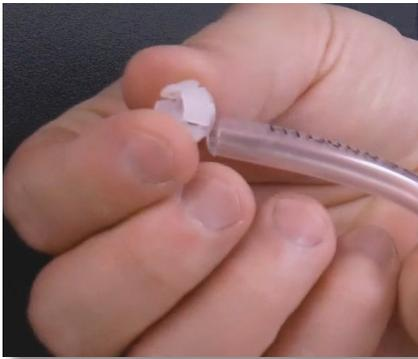
**Step 49:** Slide the collar back onto the tube, and make sure the collar's crown is pointing away from the tube nut.
