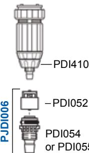
**NOTE #2:** If only the check valve barb (PDI054 or PDI055) comes out, take a pencil (eraser side down), put through the top of the injection stem assembly and gently push the check valve guide (PDI052) out.
