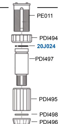
**!** To remove o-ring easily without tools, squeeze it on either side to raise the seal, then slide it over the groove
