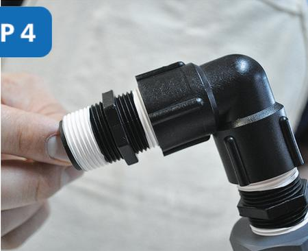
Attach the other **2" nipple** to the other side of the **elbow**.
