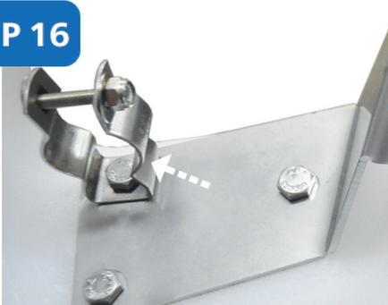
Take the hose support clamp provided in the hook-up kit. Place the last bolt through the hole on the hose support clamp and then through the remaining hole on the bracket.
