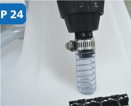
To attach the injection pickup hose to the Dosatron, place the strainer onto the hose and drop into the top of the cart tank. Thread the hose up through the hole on the top and attach a clamp to the hose. Thread the hose and clamp onto the Dosatron barb. Tighten clamp with a flat head screwdriver.
