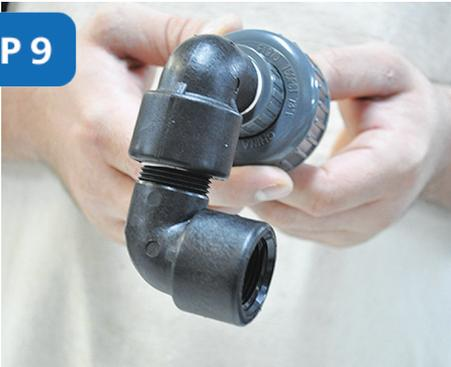
Attach the other **street elbow** to the end of the elbow and turn to a 90° angle, as shown.
