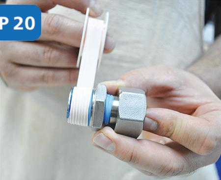
Wrap **thread seal tape** around the threads of the **stainless steel hose adapter** supplied with the cart.
