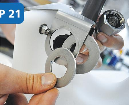
Install the **stainless steel adapter** parts by placing one washer on the inside of the cart bracket and one on the outside. Thread the stainless steel hose adapter onto the elbow and tighten with a box crescent wrench for a snug fit.
