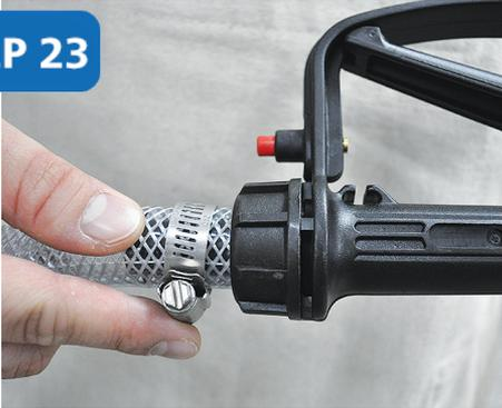
Place the **hose clamp** over the other end of the **hose** and attach to the **gas style nozzle**. Tighten the **hose clamp** with flat head screwdriver.
