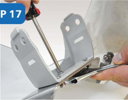
Attach the **Dosatron bracket** to the cart using the screws included on the cart.
