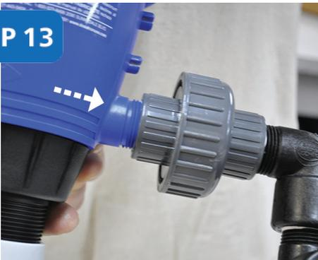
Pick up the **outlet assembly** and attach the **union** to the outlet side of the Dosatron. Note the direction of the arrow. Hand tighten.
