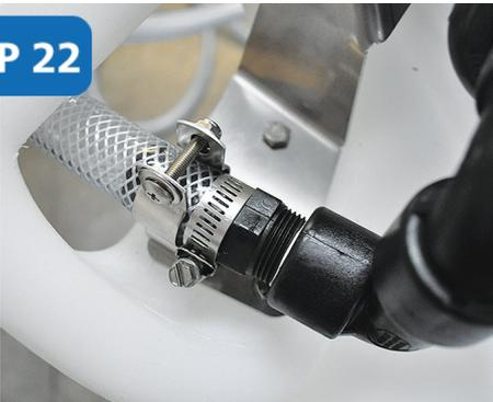
To install the **hose** onto the **hose barb**, place the **hose clamp** over **hose**. Spread support clamp on cart and attach hose with clamp onto the **hose barb**. Tighten clamp with flat head screw driver. Using a Phillips head screwdriver, tighten support clamp using hardware provided with cart.
