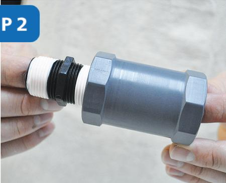
To assemble the inlet side, hold the **flow restrictor** in one hand and attach a **2" nipple** to the other side.
