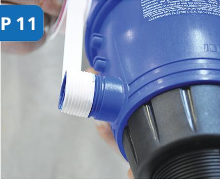
Before installing the assemblies, thread the inlet and outlet of the Dosatron with **thread seal tape**.
