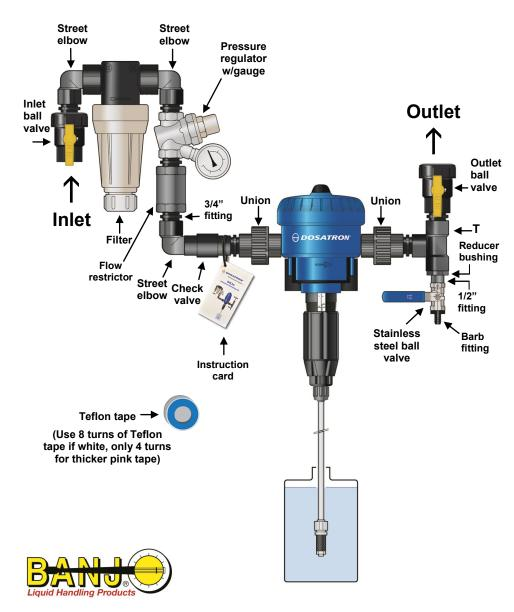
When connecting a DOSATRON either to the public water supply or to its own water source, you must respect the regulations in force concerning protection of the source i.e. backflow prevention, etc.
