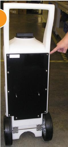
Remove the 10 screws from the back plate, to remove from the back of the DosaCart.
