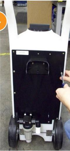
Re-attach the black plate back onto the DosaCart by installing eight screws around the plate except for the top two screws (these will be used for the crash bar, see step 9).
