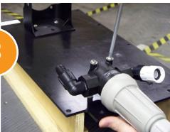
Attach the 200 mesh/80 micron filter to the bottom left of the back of the plate.
