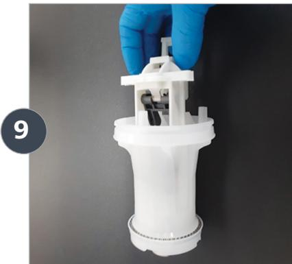
Grasp the top of the white plastic components inside the piston shell, and pull the piston's mechanism up and out.
