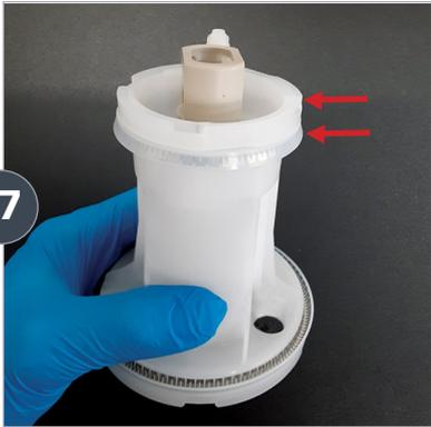
Flip the piston shell over and repeat step 15 - 16 to install the **NEW Lower Piston Flange (MPDI244U)** and **Lower Locking Ring (PDI1237)**.
