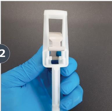
Install the **NEW Omega Spring (PDI651U)** by carefully pushing into its location on the push rod. You will hear a small click when secured properly.
