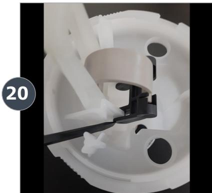
To demonstrate the alignment of the push rod assembly, the curved top would be facing inward, inserting the push rod into the single hole at the bottom of the piston shell.
