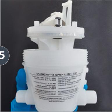
Carefully press the piston back into the injector and reinstall the bell housing.
