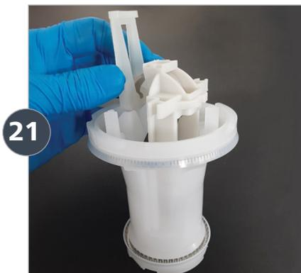
To insert both the valve support frame and the push rod into the piston shell, use your index finger to push on the spring.
