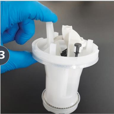
To test the piston, pull the push rod up then push down a few times, it should click in both directions.
