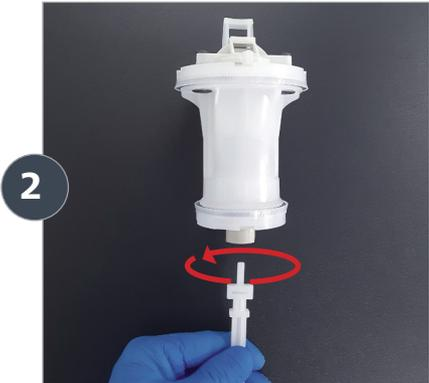
Remove the Plunger from the Piston by twisting a quarter turn counterclockwise, and set aside.
