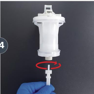
Reinstall the plunger into the bottom of the piston shell and twist a quarter turn clockwise to lock into place.
